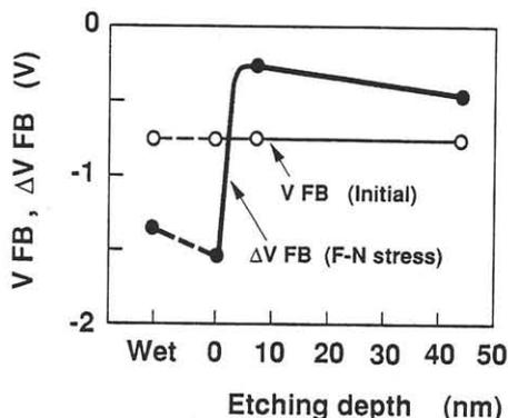
Fig.3. Photo etching depth dependence of flat band voltage ( $V_{FB}$ ) at the initial state and flat band voltage shifts ( $\Delta V_{FB}$ ) during Fowler-Nordheim injection.
