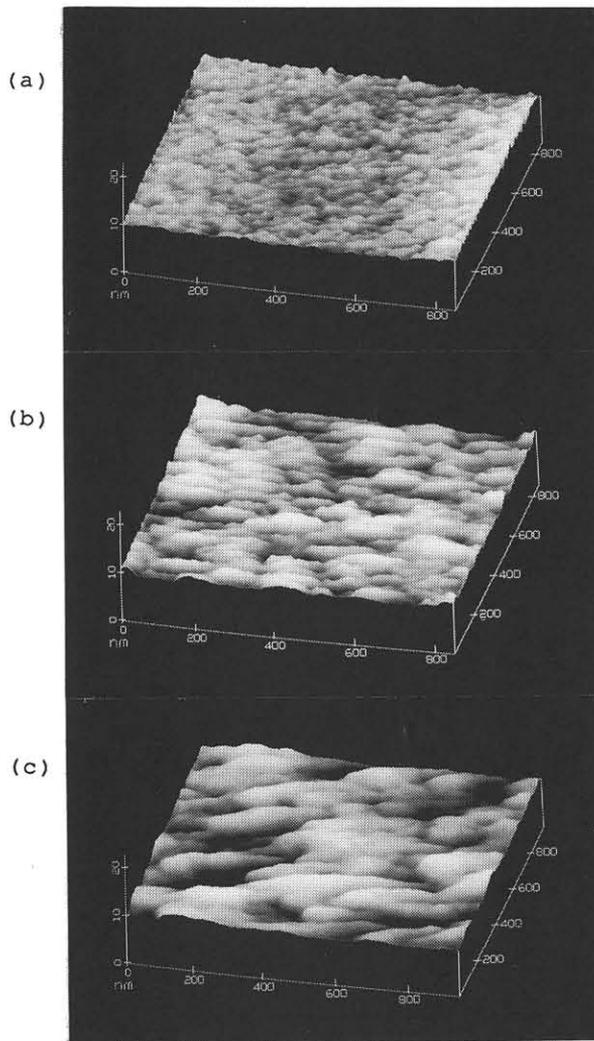
Fig.5. Si surfaces images by STM after wet cleaning(a), 6 nm(b) and 44 nm(c) photo-excited etching.
