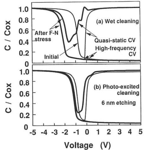
Fig.1. High-frequency and quasi-static C-V curves before and after Fowler-Nordheim current injection.
