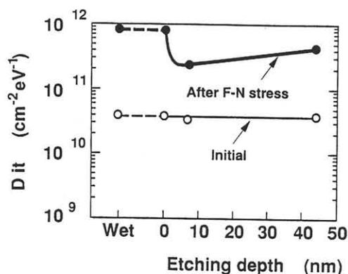
Fig.4. Photo etching depth dependence of interface state density ( $D_{it}$ ) before and after Fowler-Nordheim injection.
