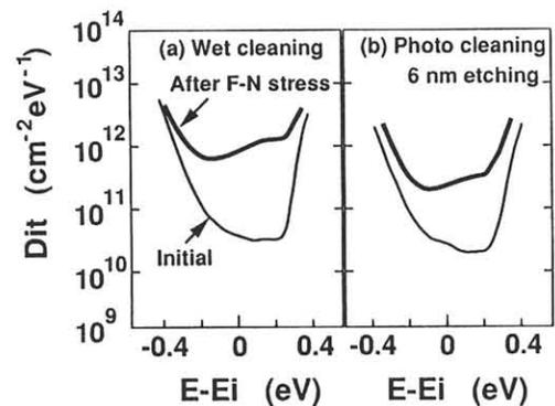
Fig.2. Interface state distribution before and after Fowler-Nordheim current injection for wet (a) and photo (b) cleaning.
