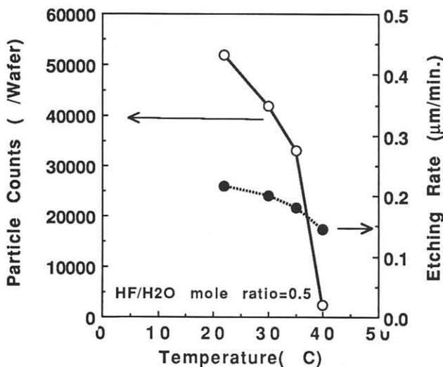
Fig.5 Wafer temperature dependence of particle counts
