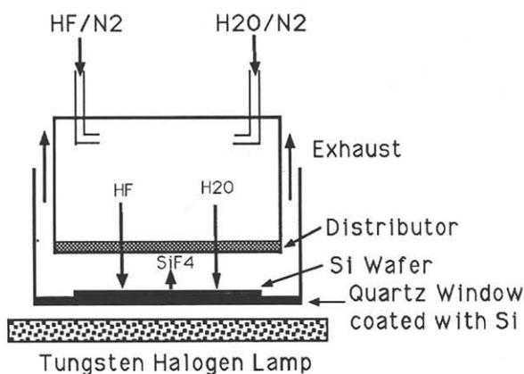
Fig.1 Schematic drawing of the etching chamber used in this experiment.
