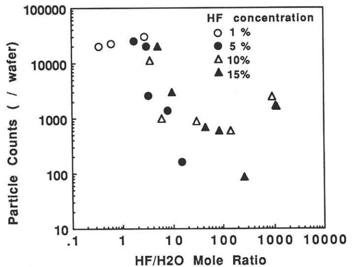
Fig.3 HF/H<sub>2</sub>O mole ratio dependence of the particle counts
