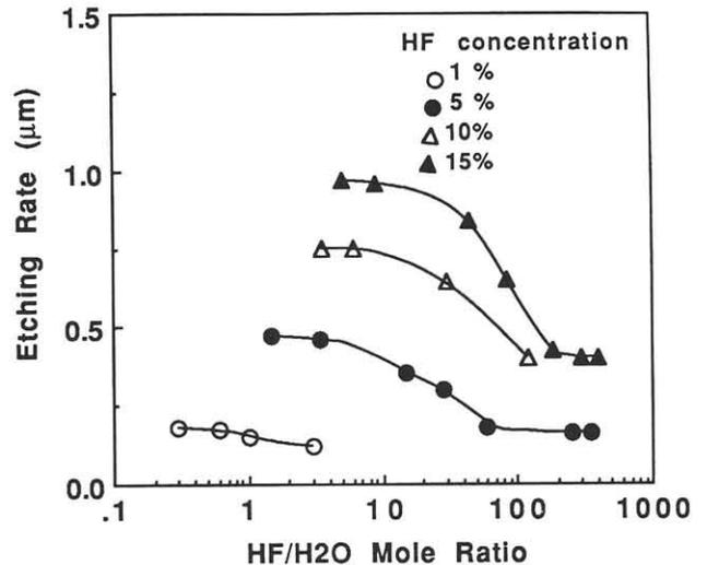
Fig.2 HF/H<sub>2</sub>O mole ratio dependence of the etching rate at various HF concentration
