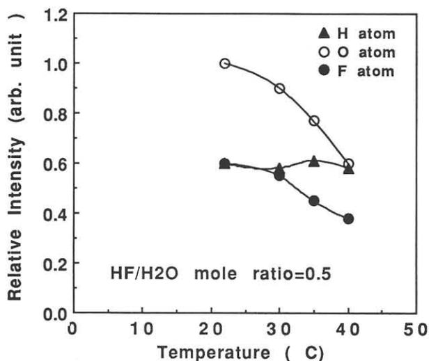
Fig.6 Wafer temperature dependence of relative intensity of H, O, and F atom
