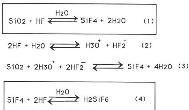
Fig.7 Reaction mechanism between SiO<sub>2</sub> film and HF/H<sub>2</sub>O gas
