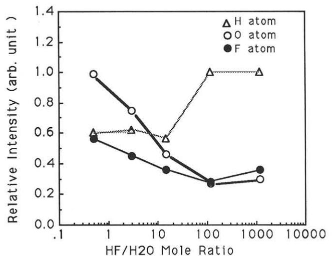
Fig.4 HF/H<sub>2</sub>O mole ratio dependence of H, O, F atom intensity
