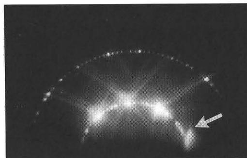
Fig. 1. RHEED pattern from vicinal Si(111) surface misoriented  $6^\circ$ . Incident azimuth is parallel to step edge ( $[\bar{1}10]$  incidence). Additional streak is indicated by arrow.
