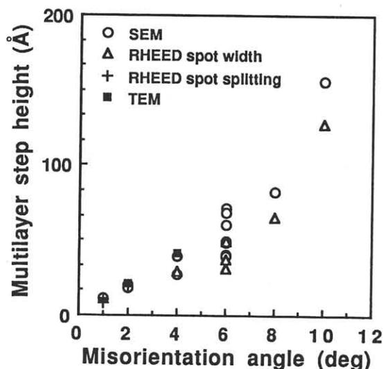
Fig. 5. Misorientation angle dependence of multilayer step height on vicinal Si(111) surface.
