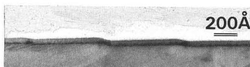
Fig. 4. Cross-sectional TEM image of vicinal Si(111) surface misoriented 2° with  $\alpha$ -Ge cap layer thickness of about 20 Å.
