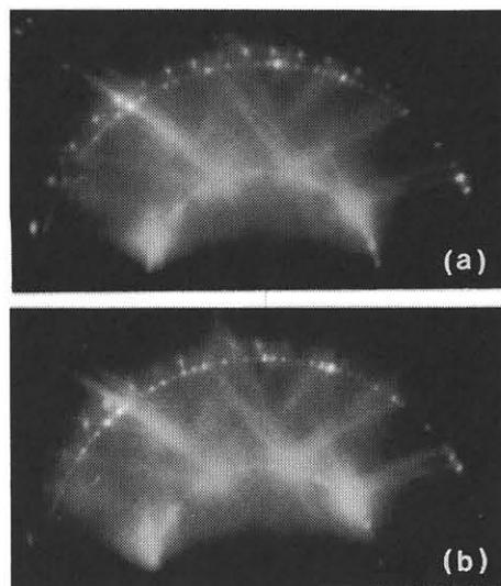
Fig. 7. RHEED patterns from vicinal Si(111) surfaces misoriented 10°. (a) cooling rate from 710°C to 550°C is 0.5(K/sec), (b) 6(K/sec).
