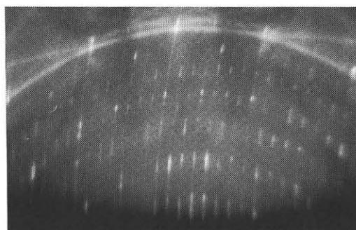
Fig. 3. RHEED pattern from vicinal Si(111) surface misoriented  $6^\circ$ . Incident azimuth is  $30^\circ$  from  $[1\bar{1}0]$  to  $[1\bar{1}2]$ .
