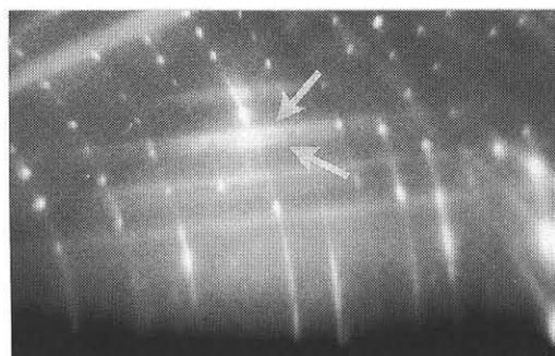
Fig. 2. RHEED pattern from vicinal Si(111) surface misoriented  $6^\circ$ . Incident azimuth is  $12^\circ$  from  $[1\bar{1}0]$  to  $[1\bar{1}2]$ . A pair of 444 Kikuchi lines are indicated by arrows.
