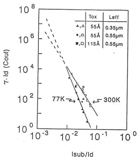
Fig. 4 Relationship  $\tau I_d$  vs.  $I_{sub}/I_d$ . The slope corresponds to  $(\phi_{it}/\phi_{th}) / (w_{int}/w_{max})$ .
