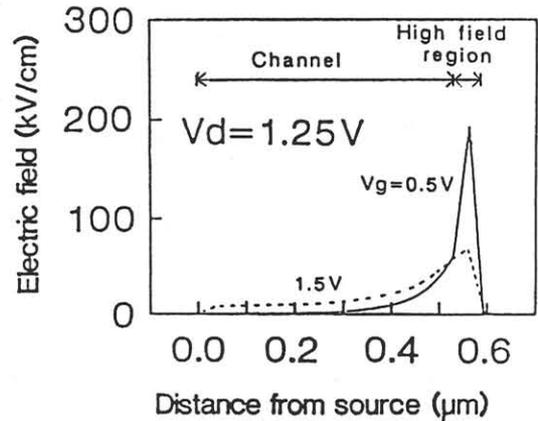
Fig. 2 Simulated lateral electric field along electron path. The bias condition is  $V_d=1.25V$ . Since electric field is rapidly changing in high field region, non-steady state effects is significant here.
