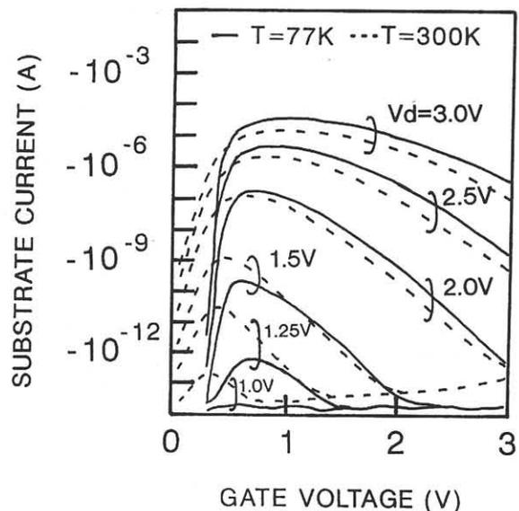
Fig. 1 Substrate current characteristics measured at 77K and 300K for nMOSFET with  $T_{ox}=55\text{Å}$  and  $W_{eff}/L_{eff}=45\mu\text{m}/0.55\mu\text{m}$ . When supply voltage is lower than 1.5V,  $I_{sub}$  at 77K is lower.
