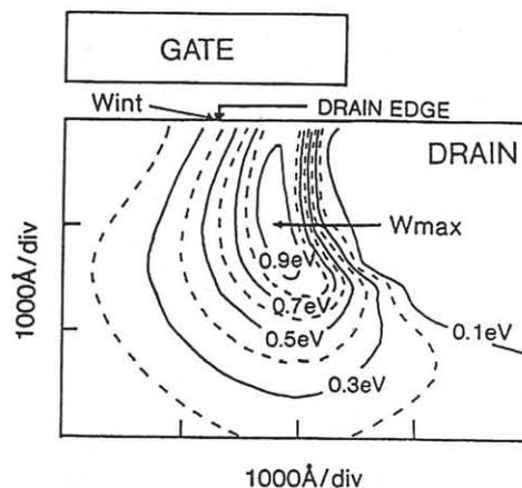
(a)  $T=77\text{K}, V_d=4.0\text{V}, V_g=1.5\text{V}$
