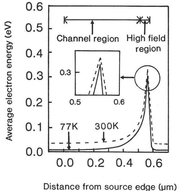
Fig. 3 Simulated average electron energy distribution along electron path. The bias condition is  $V_d=1.25V$  and  $V_g=0.5V$ . Maximum average electron energy is lower at 77K than at 300K due to lower initial energy at 77K and non-steady state effects in high field region.
