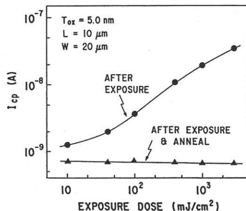
Fig. 1 Charge pumping current vs. exposure dose.
