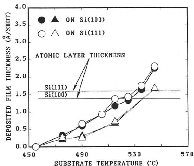
Fig.4 Substrate temperature dependence of the thickness per shot for Si films deposited using  $\text{SiH}_4$ . The shot to shot time interval was 20sec, the  $\text{SiH}_4$  partial pressure 13Pa, and the total pressure ( $\text{SiH}_4 + \text{H}_2$ ) 280Pa. Circles and triangles indicate the samples deposited with and without flash lamp light shots, respectively.
