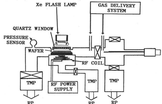
Fig.1 Schematic diagram of an ultraclean RF-heated cold-wall LPCVD system with Xe flash lamp.
