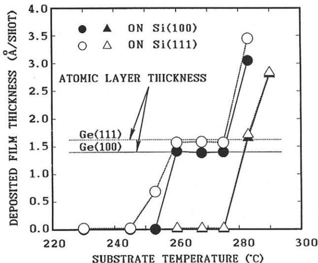
Fig.2 Substrate temperature dependence of the thickness per shot for Ge films. The shot to shot time interval was 20sec, the  $GeH_4$  partial pressure 13Pa, and the total pressure ( $GeH_4 + H_2$ ) 280Pa. Circles and triangles indicate the samples deposited after a 400°C pre-heating and without a 400°C pre-heating, respectively.
