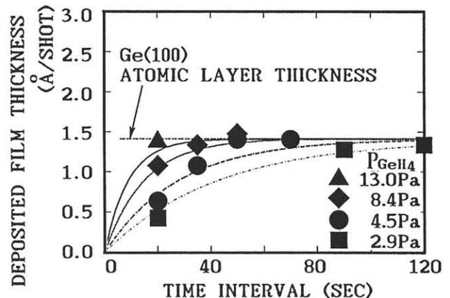
Fig.3 Shot to shot time interval dependence of deposited Ge thickness per shot for various  $GeH_4$  partial pressures on a Si(100) substrate at a substrate temperature of 268°C.
