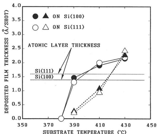
Fig.5 Substrate temperature dependence of the thickness per shot for Si films deposited using  $\text{Si}_2\text{H}_6$ . The shot to shot time interval was 20sec, the  $\text{Si}_2\text{H}_6$  partial pressure 100 Pa, and the total pressure ( $\text{Si}_2\text{H}_6 + \text{H}_2$ ) 300 Pa. Circles and triangles indicated the samples deposited with and without flash lamp light shots, respectively.
