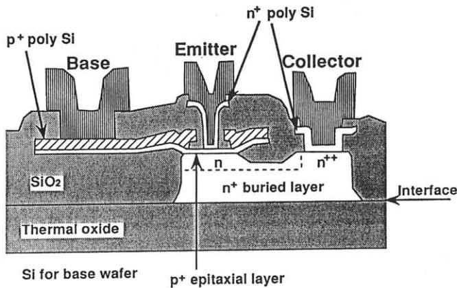
Fig. 5. Cross section of the EBT fabricated on SOI.
