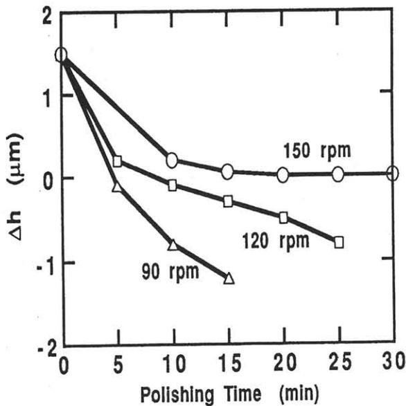
Fig. 2. Polishing time and work revolution dependence of Si island thickness. The difference in the height between the Si island and stopper is indicated by  $\Delta h$ .
