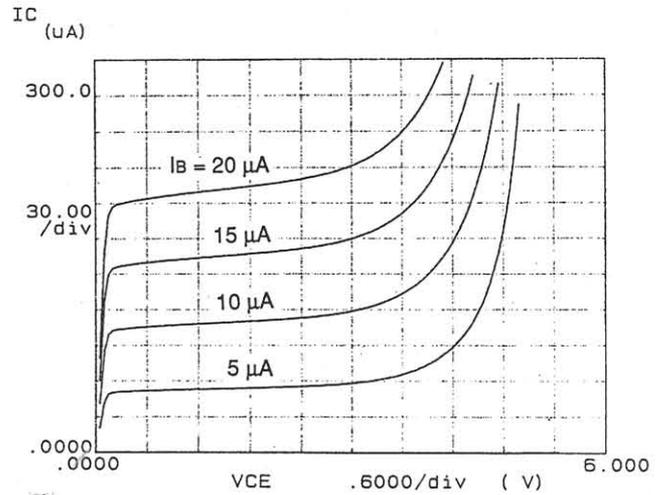
Fig. 6. I-V characteristics of the EBT on SOI.
