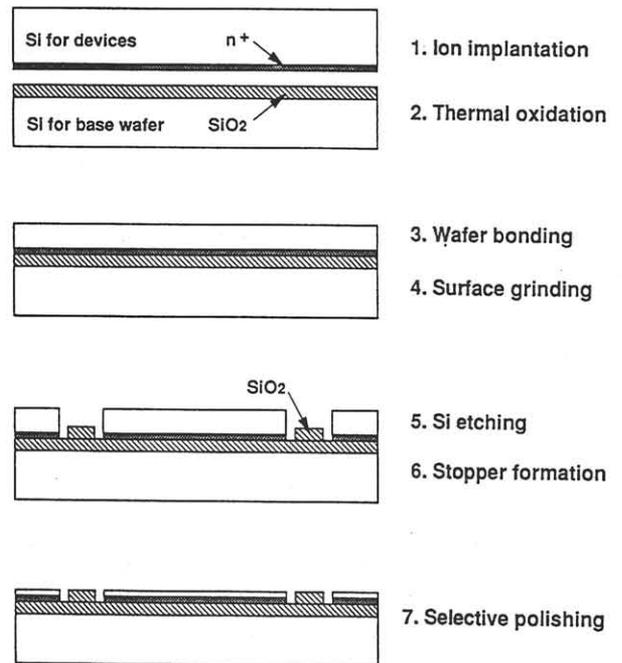
Fig. 1. Wafer bonding and selective polishing for the SOI with n<sup>+</sup> buried layer.
