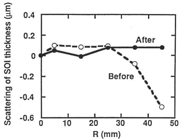
Fig. 3. Scattering of SOI thickness before and after selective polishing. The distances from the center of the wafer are indicated by R.
