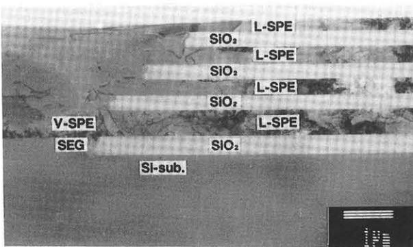
Figure 4 Cross-sectional TEM view of a 5-layer-stacked structure
