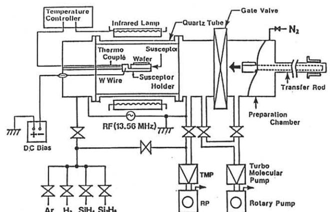
Figure 1 Schematic diagram of the apparatus for the U-LPCVD
