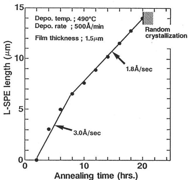
Figure 2 Annealing time dependence for L-SPE length for an a-Si film on a thin SiO<sub>2</sub> layer
