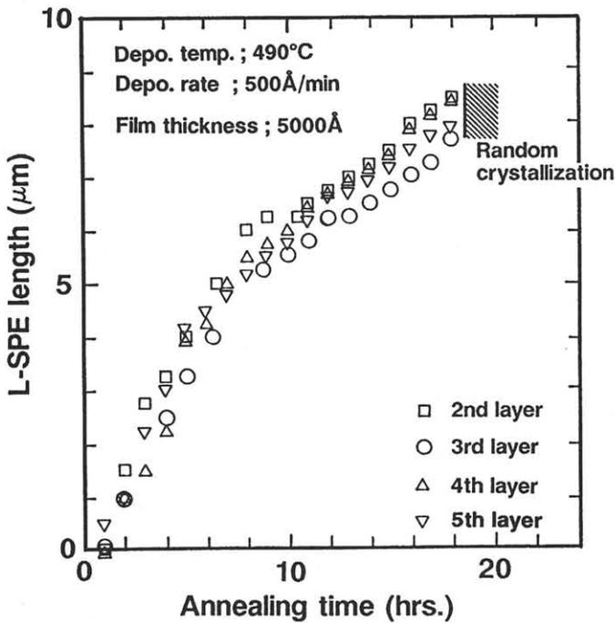
Figure 5 Annealing time dependence of L-SPE length for each layer
