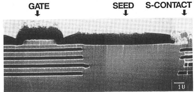
Figure 6 Cross-sectional SIM view of an n-MOS FET fabricated onto a top layer
