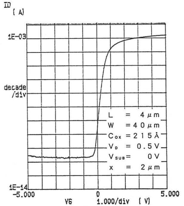
Figure 7 Typical  $I_D$ - $V_G$  characteristics for an n-MOS FET fabricated on a top layer
