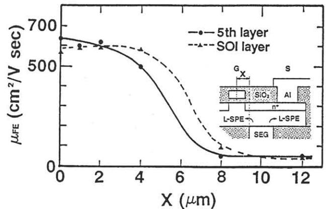
Figure 8 Dependence of  $\mu_{FE}$  on gate distance, ( $X$ ), away from the edge of an seeded window
