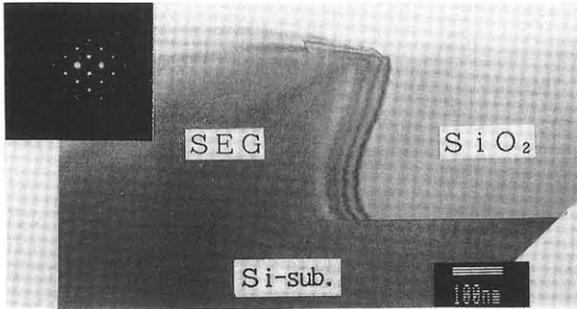
Figure 3 Cross-sectional TEM view of an SEG layer
