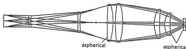
Figure-8 The newly designed aspherical lens system with 15mm-square and NA0.45.
