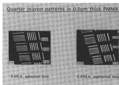
Figure-9 SEM photographs of 0.23 micron to 0.30 micron patterns in 0.5 micron thick PMMA ; (a) spherical lens, (b) aspherical lens.
