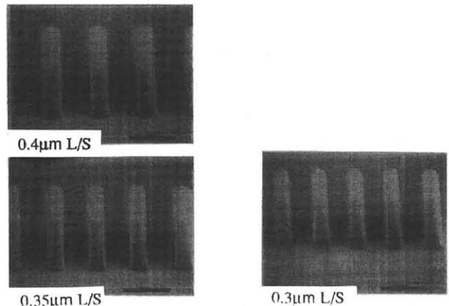
Figure-1 SEM photographs of 0.4 micron down to 0.3 micron line and space pattern ASKA2, thickness of 1.0 micron, on Si substrate by exposed KrF excimer laser stepper with NA 0.42.
