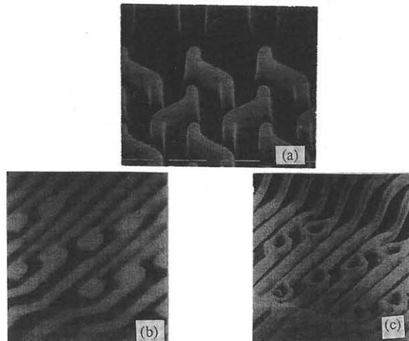
Figure-7 SEM photographs of the demonstrated pattern for a proto-type 64MDRAMs: (a) isolation pattern on SiN/SiO<sub>2</sub>, (b) connection pattern on TiN/AlSiCu, (c) connection pattern after etching.
