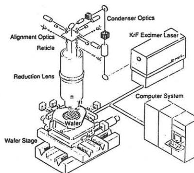
Figure-6 Schematic diagram of the TTR alignment system.
