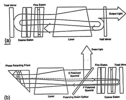
Figure-4 Schematic representation of spectral narrowing lasers with intra cavity etalons: (a) a conventional laser, (b) a new laser polarization coupled resonator.
