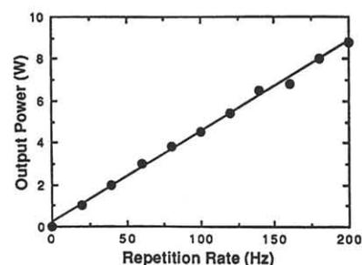
Figure-5 Output power vs.repetition rate in the new PCR laser.
