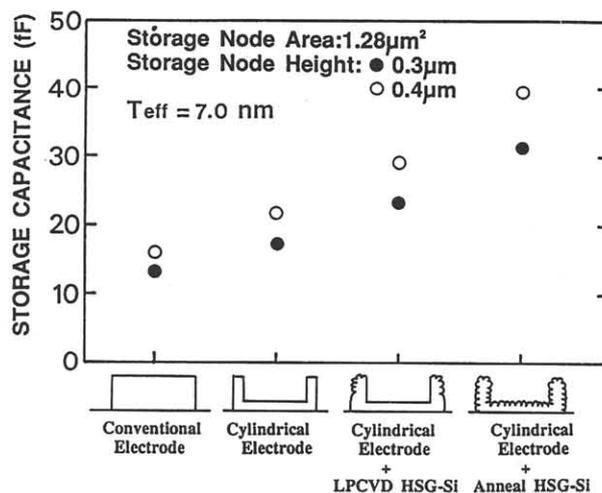
Fig.4 Storage capacitances for various electrode structures for 64Mbit DRAM.
