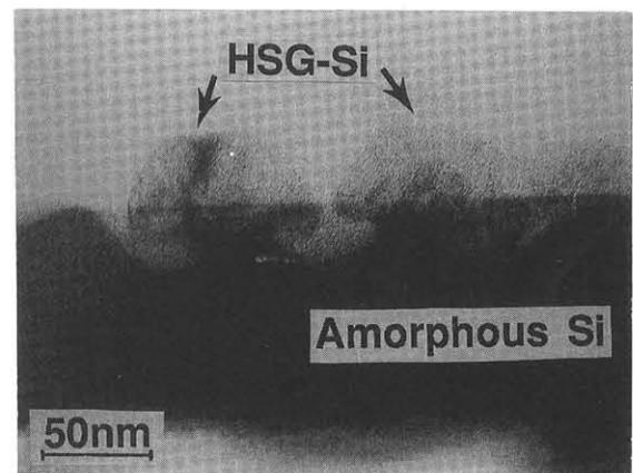
Fig.2 Cross-sectional TEM micrograph of a Si film annealed in a high vacuum.
