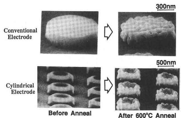
Fig.3 SEM photographs of two types storage electrodes before and after high-vacuum annealing.
