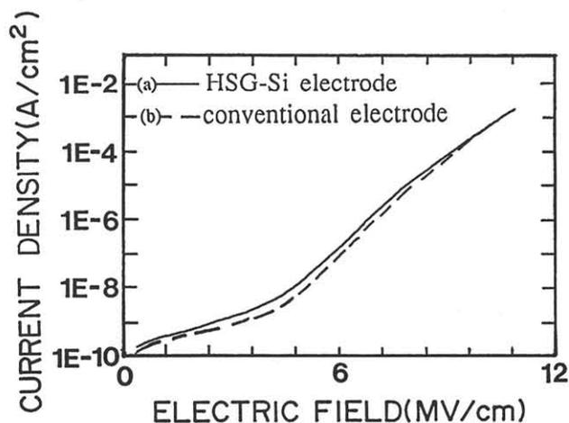
Fig.5 I-E characteristics of 7nm(Teff)- $\text{SiO}_2/\text{Si}_3\text{N}_4$  dielectric films formed on annealing-method HSG-Si electrodes and conventional electrodes.
