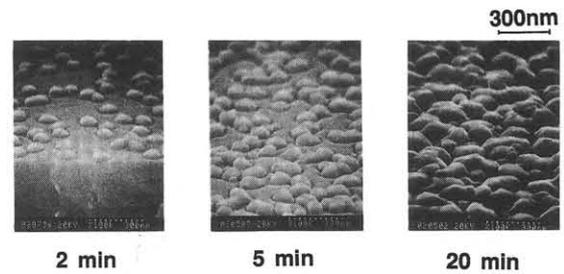
Fig.1 SEM photographs of Si film surface morphology depending on the holding time after deposition in a vacuum at 590°C.
