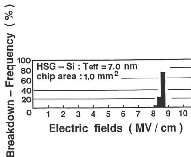
Fig.6 Breakdown field distribution of  $T_{eff}=7\text{nm}$ ( $T_{eff}$ )- $\text{SiO}_2/\text{Si}_3\text{N}_4$  films on annealing method HSG-Si electrodes.
