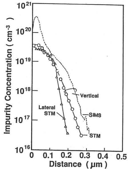
Fig.2 Impurity concentration profiles. Lateral profile was measured beneath the mask starting from the edge.
