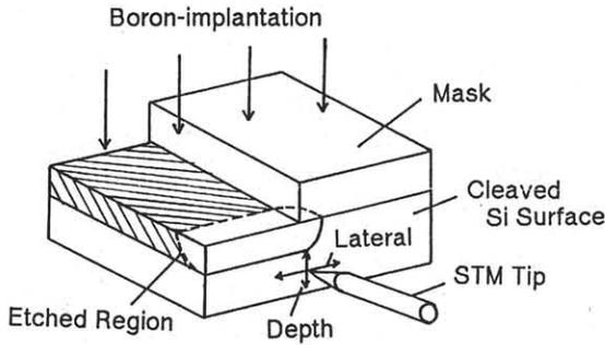
Fig.1 Schematic drawing of the proposed implant dopant profiling method using STM.
