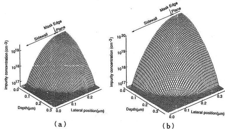
Fig.3 Two-dimensional impurity profiles obtained with (a)STM and (b)SIMS.
