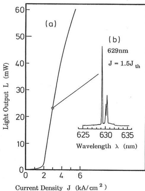
Fig.6. Light output versus injected current density (a) and lasing spectrum (b) of the GaInP/AlInP MQW-SLC LDs.
