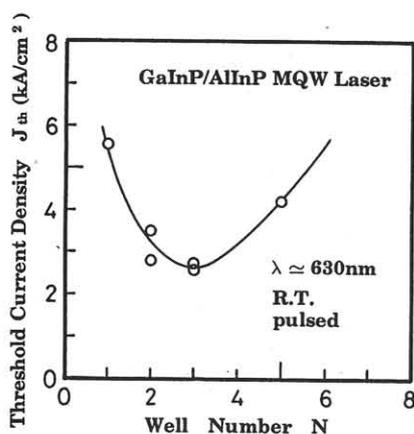
Fig.5. The threshold current density versus well number for GaInP/AlInP MQW lasers.
