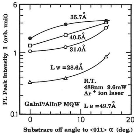
Fig.2. PL peak intensity as a function of the substrate off angle for GaInP/AlInP MQW active layers with various well widths.
