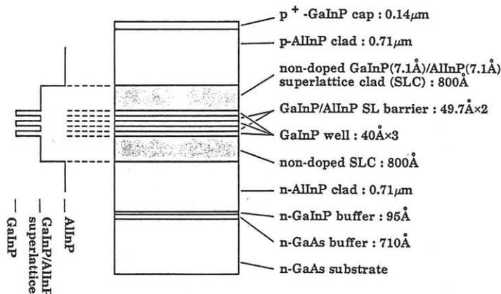
Fig.1. Schematic diagram of 630nm GaInP/AlInP MQW-SLC LDs.
