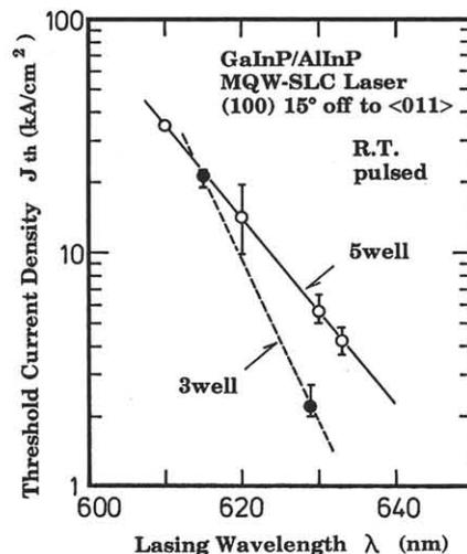
Fig.4. Lasing wavelength dependency of the threshold current density of five-QW type lasers.
