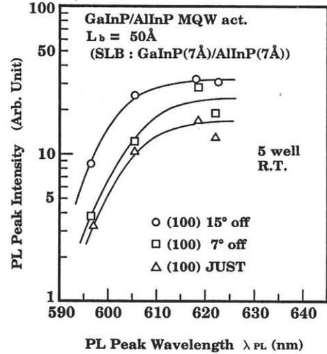
Fig.3. PL peak intensity from GaInP/AlInP MQWs as a function of PL peak wavelength.
