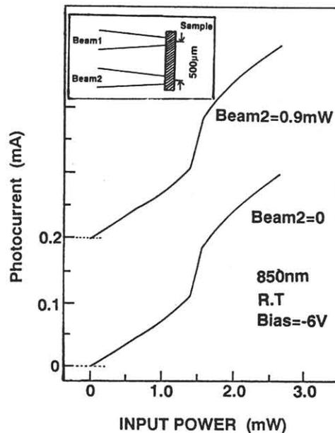
Figure 3 Photocurrents as a function of the incident light power of the Beam1 at room temperature. The upper and lower curves correspond to the case with two beams spatially separated by a distance of  $\sim 500 \mu\text{m}$  and the case with the only one beam (Beam1), respectively.
