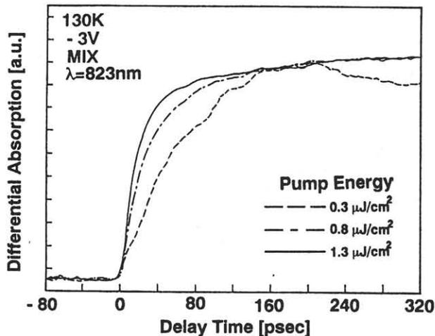
Figure 1 Time-resolved differential absorption for different optical input powers obtained by a pump-probe measurement performed with 6 psec.-optical pulses.
