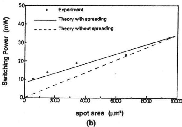
Figure 4 (a) Photocurrents as functions of the incident light power at room temperature for different beam spot sizes. (b) Dots show the experimental results on the optical switching power as a function of a beam spot area. A dashed and solid lines show theoretical results on the optical switching power as a function of a beam area without and with in-plane carrier spreading, respectively.
