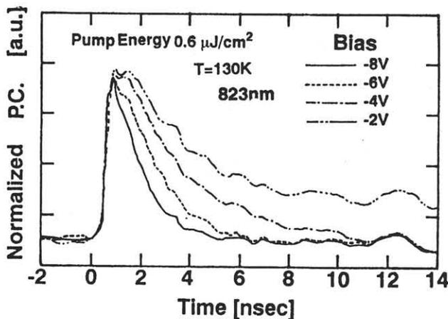
Figure 2 Time-resolved photocurrents for the different reverse bias.
