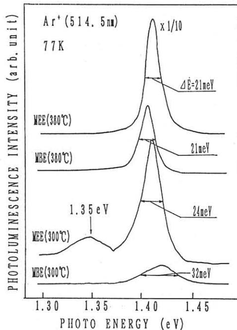
**Fig.3** PL spectra of MEE and MBE samples grown at 300°C and 380°C. A peak appears at 1.35eV in the 300°C MEE sample.
