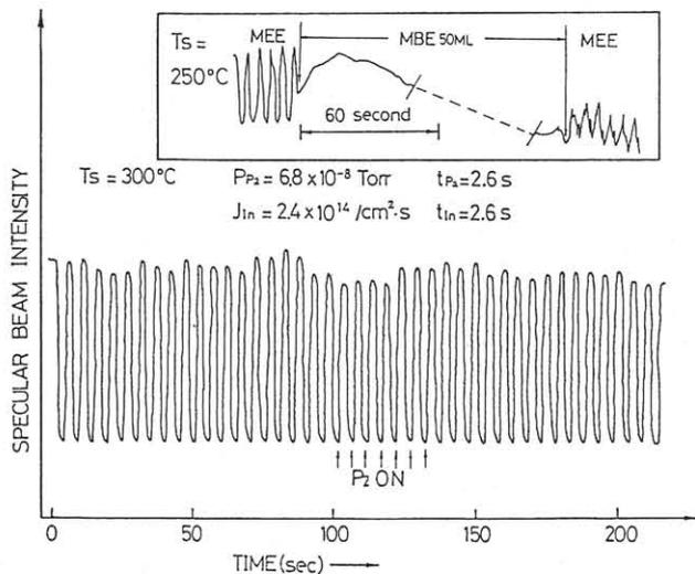
**Fig.2** RHEED specular beam intensity oscillation during the MEE growth at 300°C. The inset shows the insertion of MBE mode in the MEE growth at 250°C.
