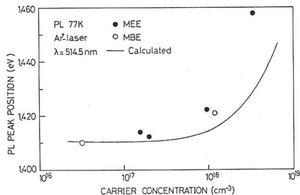
**Fig.4** Dependence of PL peak-position on carrier concentration at 77K. Solid line is the calculated result based on the theory<sup>(6)</sup>.
