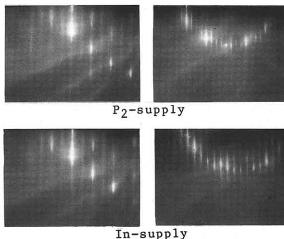
**Fig.1** RHEED patterns from (001) InP surface during MEE growth. Left side from the [110] azimuth and right from the [1 $\bar{1}$ 0].
