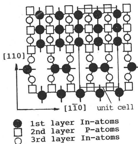
Fig.5 A new model for the In-stabilized InP (001)-surface of (2x4) structure.
