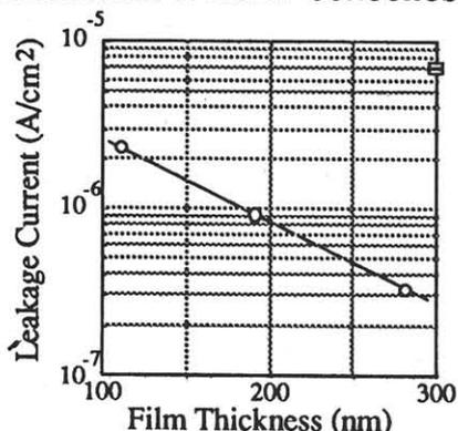
Fig.6 The dependence of the leakage current on the film thickness measured at the bias condition of 1.65V;  $\circ$ : the PLZT films having lanthanum 5 mol%,  $\square$ : the PZT film having no lanthanum.
