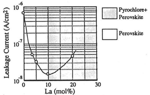
Fig.3 The dependence of the leakage current of 300nm thick PLZT film on the lanthanum concentration which is measured at the bias condition of 1.65V.
