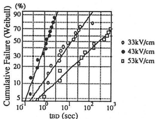
Fig.7 The time dependent dielectric breakdown of PLZT film having lanthanum 5 mol% content under the various stress conditions.
