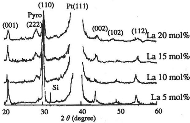
Fig.1 The X-ray diffraction pattern of PLZT films with various lanthanum concentration.
