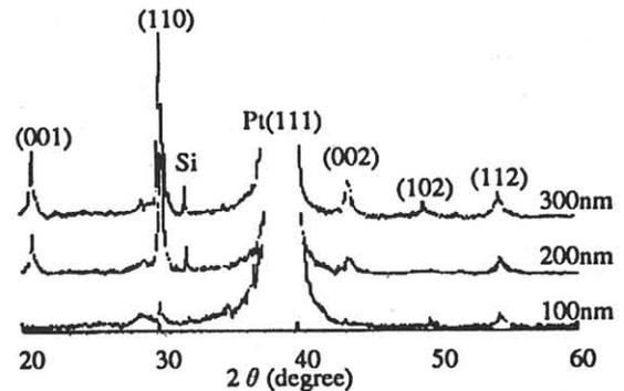
Fig.4 The X-ray diffraction pattern of PLZT films with various film thickness which content 5 mol% lanthanum.
