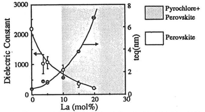
Fig.2 The relationship between the lanthanum concentration and the relative dielectric constant of 300nm thick
