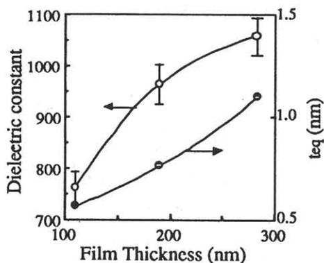
Fig.5 The relative dielectric constant versus thickness of PLZT films having lanthanum 5 mol% contents.
