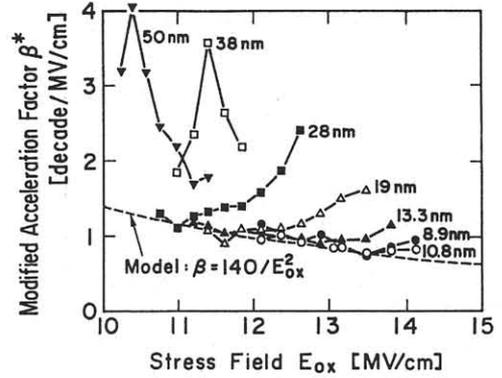
Fig.5 Acceleration factor, deduced from modified time to breakdown
