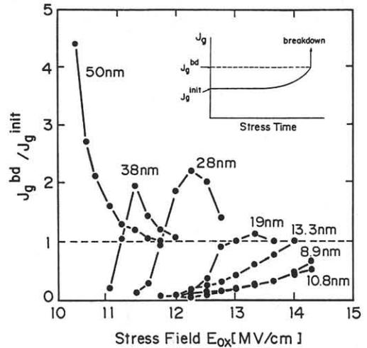
Fig.6 The ratio of current density at the initial stress point and at the breakdown point for various stress conditions
