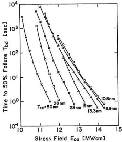
Fig.2 Time to breakdown versus stress field strength
