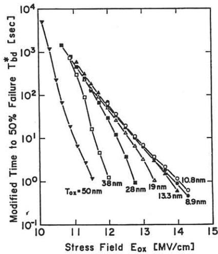
Fig.3 Modified time to breakdown versus stress field strength
