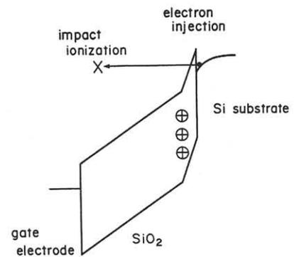
Fig.7 Diagram showing effective potential versus distance from the Si/SiO<sub>2</sub> interface
