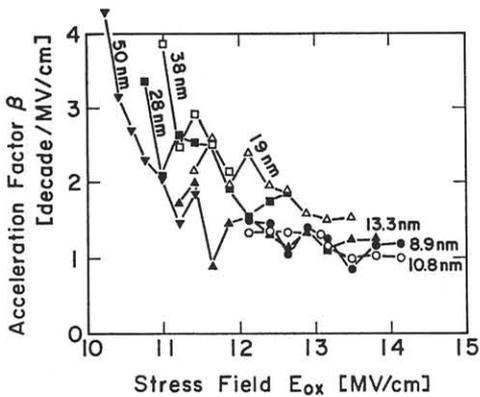
Fig.4 Acceleration factor versus stress field for various oxide thicknesses
