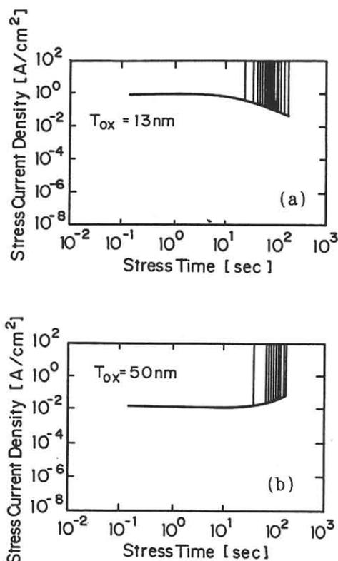
Fig.1 Stress current shift during constant voltage stress for (a) 13 nm and (b) 50 nm oxides
