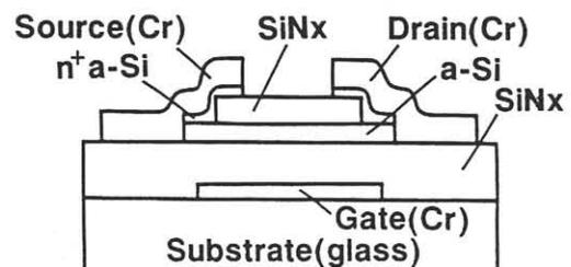
Fig.1 a-Si TFT configuration.
