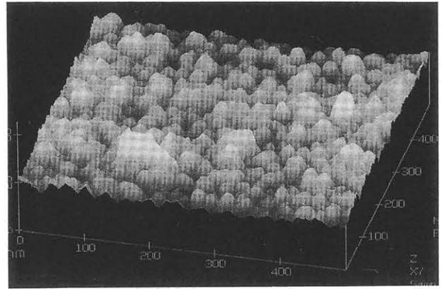
(d) 6nm thick a-Si deposited under high power conditions on smooth SiNx.
