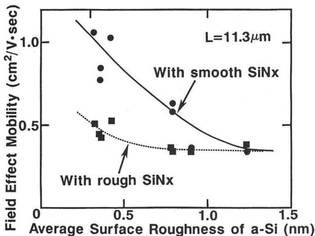
Fig.4 Field effect mobility as a function of average roughness for a-Si with smooth SiNx(0.57nm) and rough SiNx(1.62nm).
