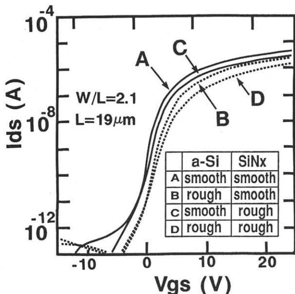
Fig.3 Transfer characteristics for TFTs.
