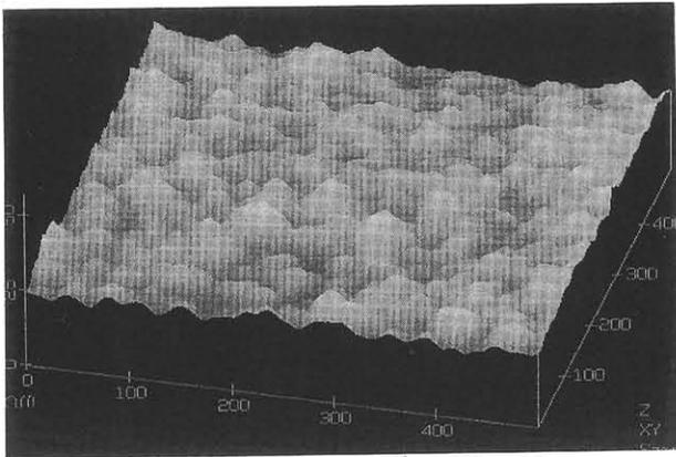
(c) 6nm thick a-Si deposited under low power conditions on smooth SiNx.
