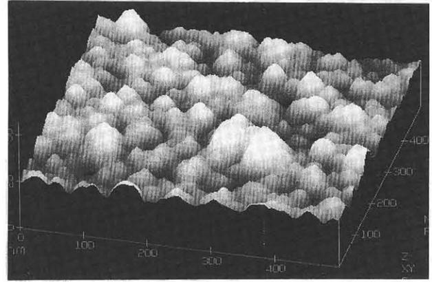
(b) SiNx deposited under rough conditions.
