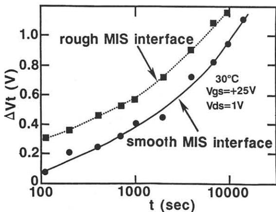
Fig.5 Threshold voltage shift as a function of time for smooth and rough MIS interfaces.
