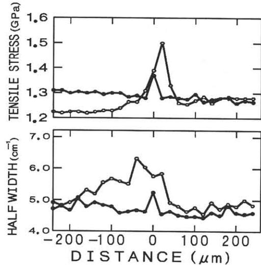
Fig.6 Tensile stress and half width measured by Raman spectroscopy of laser annealed poly-Si around first edge region.
