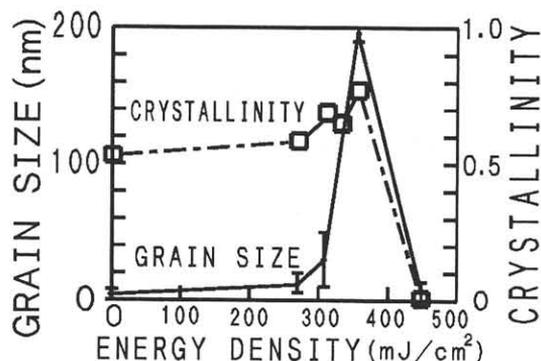
Fig.1 Grain size and crystallinity of laser annealed poly-Si dependence on laser energy density.
