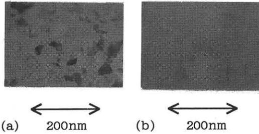
Fig.2 TEM micrograph of laser annealed poly-Si films. (a) 310mJ/cm<sup>2</sup> (b) 370mJ/cm<sup>2</sup>
