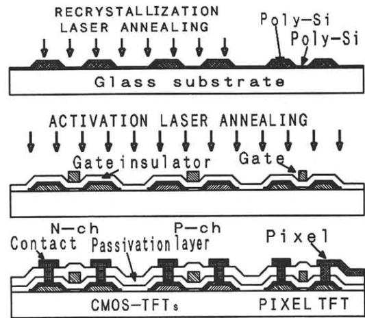
Fig.3 Process flow for self-aligned TFT with laser selective irradiation.
