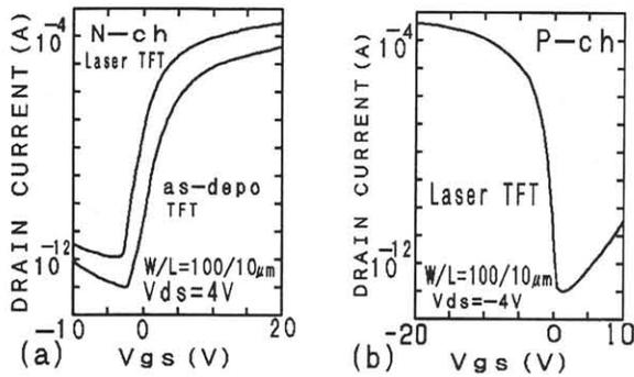
Fig.5 Drain current-gate voltage characteristics (a) n-channel and (b)p-channel of poly-Si TFT.
