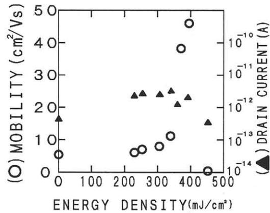
Fig.4 Mobility and off current of poly-Si TFT.
