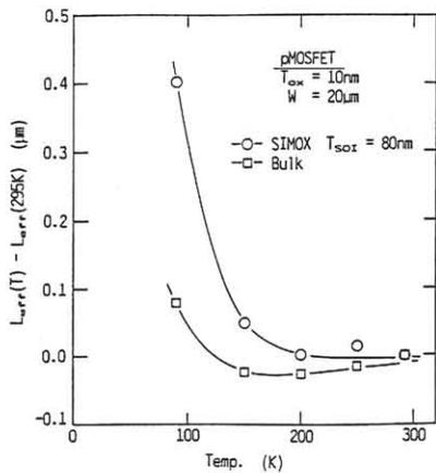
Fig. 5 Temperature dependence of effective channel length for SIMOX and Bulk pMOSFET.
