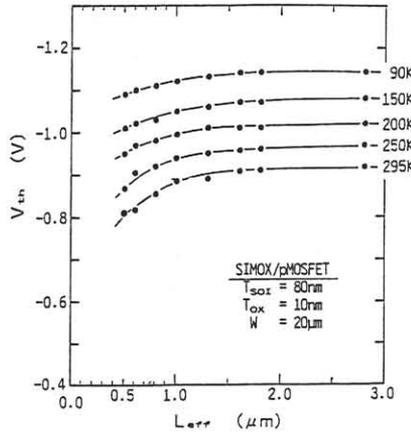
Fig. 3 Threshold voltage for SIMOX pMOSFET as a function of temperature.
