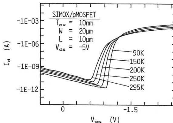
Fig. 1  $I_D$ - $V_{gs}$  characteristics as a function of temperature.
