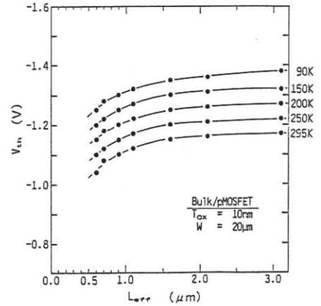
Fig. 4 Threshold voltage for Bulk pMOSFET as a function of temperature.
