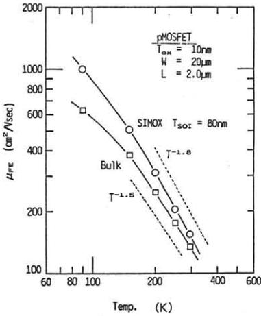
Fig. 2 Field effect mobility for SIMOX and Bulk pMOSFET.
