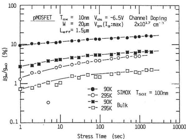
Fig. 7 Stress time variation for change of transconductance for SIMOX and Bulk pMOSFET.
