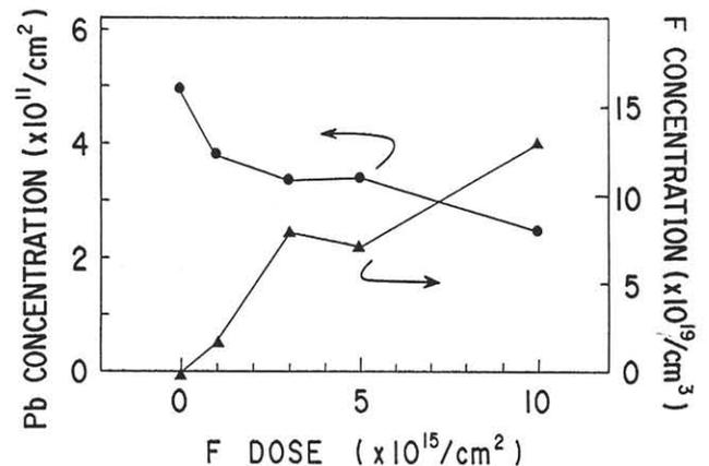
Fig.5. F dose dependence of Pb center and interface F concentrations.
