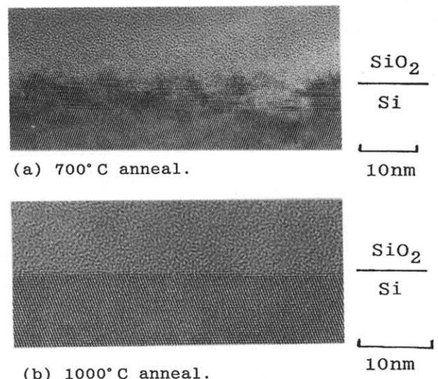
Fig.2. TEM images near the SiO<sub>2</sub>/Si interface for F dose of  $3 \times 10^{16} \text{ cm}^{-2}$ .
