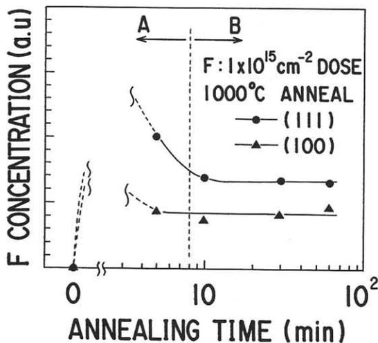
Fig.3. Interface F concentration for (111) and (100) interfaces.
