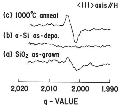
Fig.4. ESR signals of Pb center for the unimplanted samples.
