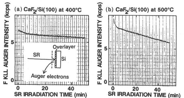
Fig. 4 Simultaneously-monitored  $F_{KLL}$  Auger signal intensity as a function of SR irradiation time at  $400^\circ C$  (a) and  $500^\circ C$  (b). Samples are  $CaF_2$  films.
