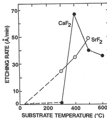
Fig. 2 Synchrotron radiation etching properties as a function of substrate temperature. Samples are CaF<sub>2</sub> and SrF<sub>2</sub> films deposited on Si(111) substrates at room temperature.
