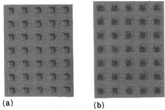
Fig. 3 SR-etched mesh patterns on  $CaF_2/Si$  at (a)  $400^\circ C$  and (b)  $500^\circ C$  for 50 min. A #2000 mesh was placed less than 1 mm above the  $CaF_2$  films. The etched area is about  $6\mu m \times 6\mu m$ .
