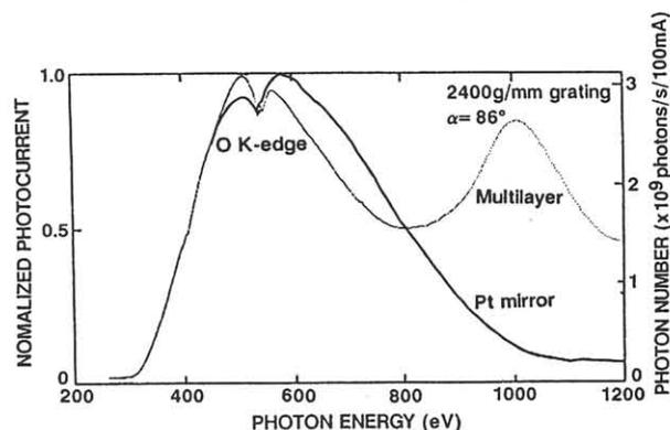
Fig. 1 Monochromatization characteristics obtained by applying a multilayer or a Pt mirror as the first optical element in the grating/crystal monochromator. The incidence angle of synchrotron radiation to the multilayer and the grating was 86°.
