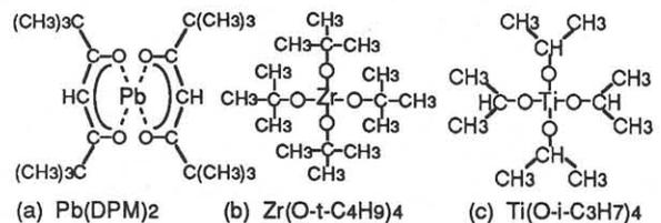
Fig.2 Metalorganic source materials for CVD-PZT.
