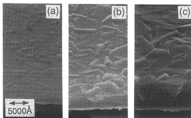
Fig.6 Surface morphology dependence on film thickness : (a)850Å (b)3500Å (c)7300Å. The deposition condition is fixed.
