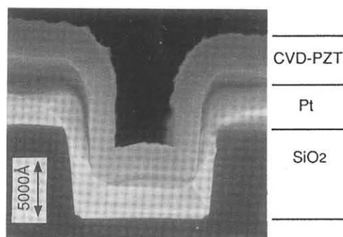
Fig.5 Cross sectional SEM photograph of step coverage of PZT over Pt step.
