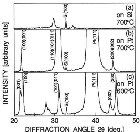
Fig.3 X-ray diffraction patterns of CVD-PZT on (a)Si(100) and (b)(c)Pt(111). The temperature of substrate is (a)700°C (b)700°C (c)600°C.
