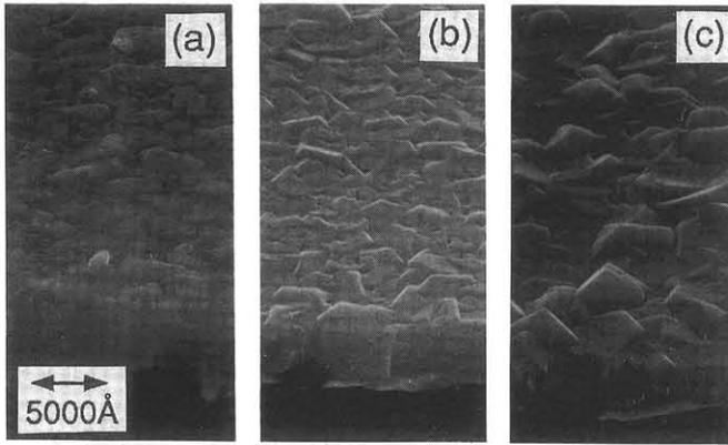
Fig.7 SEM observations of surface morphology as a function of Pb supply condition. (a)100sccm (b)150sccm (c)200sccm. Other conditions are same.
