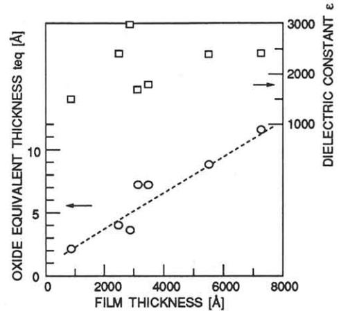
Fig.8 Oxide equivalent thickness ( $t_{eq}$ ) and dielectric constant ( $\epsilon$ ) as a function of the film thickness of PZT. The capacitance of 850Å thick PZT corresponds to 2.1Å silicon dioxide.
