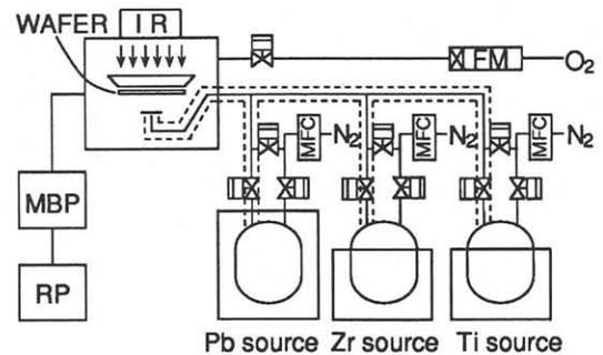
Fig.1 Schematic diagram of apparatus for CVD-PZT.
