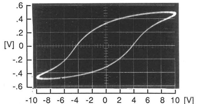
Fig.10 Characteristic P-E hysteresis loop generated using a 1kHz sine wave and an amplitude of 10V.  $Pr=18\mu\text{C}/\text{cm}^2$ , and  $E_c=55\text{kV}/\text{cm}$ . (7300Å thick, and electrode area of  $3.8 \times 10^{-3} \text{cm}^2$ ,  $C_s=0.47\mu\text{F}$ )
