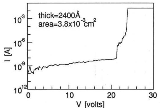
Fig.9 Leakage current(I) as a function of applied voltage(V). (2400Å thick and electrode area of  $3.8 \times 10^{-3} \text{cm}^2$ )
