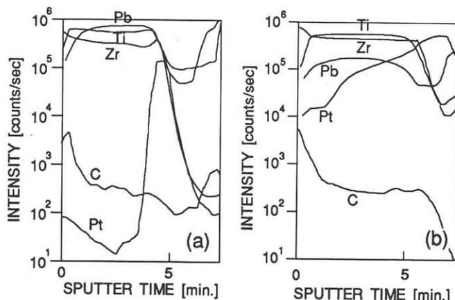
Fig.4 SIMS in-depth profile of CVD-PZT on Pt(111). The O<sub>2</sub> gas flow rate is (a)1000sccm (b)300sccm.
