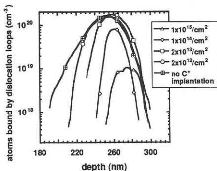
Fig.2 Profiles of atoms bound by dislocation loops near the a/c interface calculated from the cross-section TEM photographs after annealing at 600°C for 1h and at 1000°C for 75 sec for various carbon doses at 78keV.
