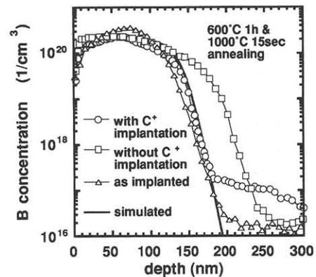
Fig.3 Boron depth profiles measured using SIMS before and after the annealing. Simulated profile after the annealing using SUPREM parameter values is also shown.
