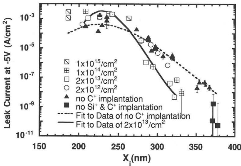
Fig.7 Junction leakage current of  $p^+/n$  junction at -5V as a function of junction depth ( $X_j$ ). Carbon ions are implanted at various doses at 78keV. Data in the case of no pre-amorphization with  $Si^+$  are also shown.
