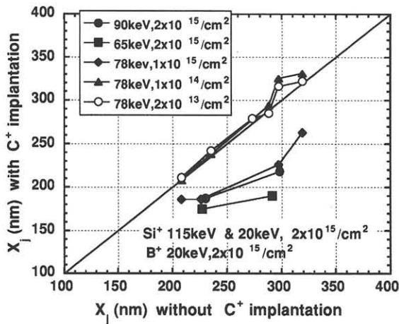
Fig.5 Junction depth( $X_j$ ) of carbon-implanted region as a function of  $X_j$  of non-carbon-implanted region for various  $C^+$  doses and energies after annealing at 950-1000°C for 15-90sec.
