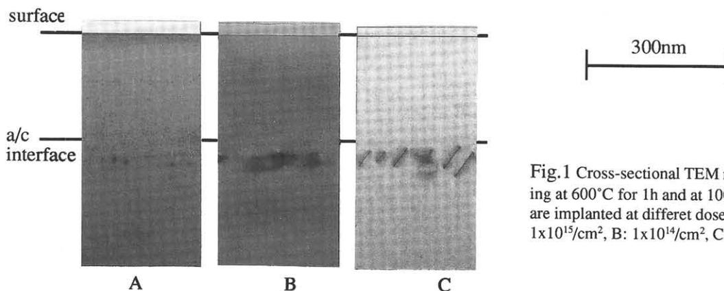
Fig. 1 Cross-sectional TEM micrographs after annealing at 600°C for 1h and at 1000°C for 75sec. Samples are implanted at different doses of C<sup>+</sup> at 78keV as; A:  $1 \times 10^{15}$ /cm<sup>2</sup>, B:  $1 \times 10^{14}$ /cm<sup>2</sup>, C: no-carbon implanted.
