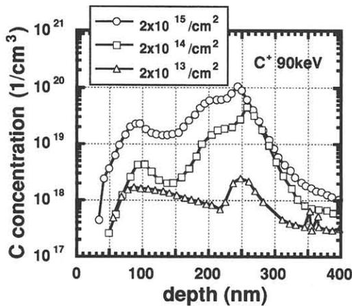
Fig.6 Carbon depth profiles after annealing at 600°C for 1h. and at 1000°C for 75sec. for various carbon doses at 90keV.
