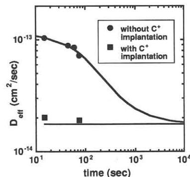
Fig.4 Annealing time dependence of effective diffusion constant ( $D_{eff}$ ) with and without carbon ion implantation at 78keV at 1x10<sup>15</sup>/cm<sup>2</sup>.
