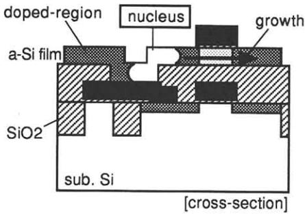
Fig. 1 Single-grain poly-Si film formation for an SRAM cell by controlling solid-phase nucleation and growth.
