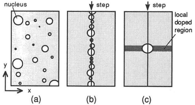
Fig. 2 Concept of solid-phase nucleation control technique. (a) random nucleation (conventional), (b) selectivity in x-direction by step-structure formatin, and (c) selectivity in y-direction by local doping.
