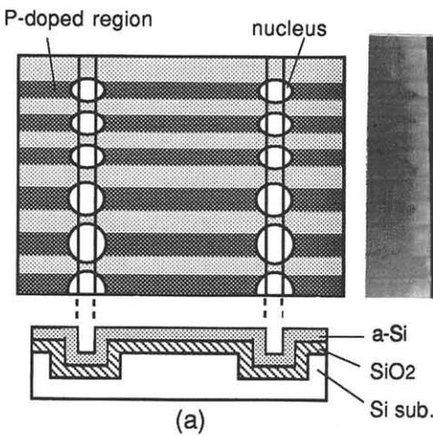
Fig. 4 Preferential nucleation induced at cross point of local P-doping region and step-structure of substrate surface. (a) sample geometry and (b) Nomarski micrograph.
