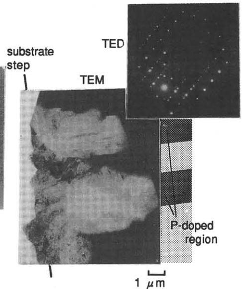
Fig. 5 TEM micrograph of nuclei shown in Fig. 4. The inset is a TED pattern of a nucleus at a cross point of the local P-doped region and the step-structure on the substrate surface.
