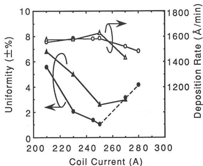
Fig. 7 Dependence of uniformity and deposition rate of SiO<sub>2</sub> on coil current. The deposition conditions are SiH<sub>4</sub> 30 SCCM, O<sub>2</sub> 30 SCCM, with a microwave power of 300W. Shape of the quartz window is plate ( $\blacktriangle, \triangle$ ) and concave ( $\bullet, \circ$ ).
