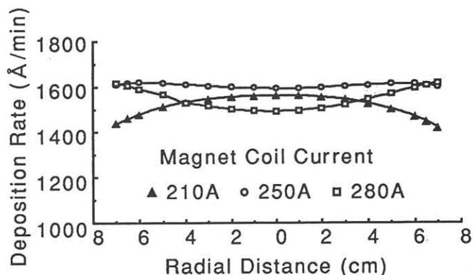
Fig. 6 Radial distribution of SiO<sub>2</sub> deposition rate. The deposition conditions are SiH<sub>4</sub> 30 SCCM, O<sub>2</sub> 30 SCCM with a microwave power of 300 W.
