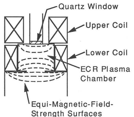
Fig. 4 Novel magnetic configuration for a concave equi-magnetic-field-strength surface near the quartz window.
