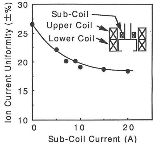
Fig. 3 Dependence of the ion-current uniformity on sub-coil current. The upper coil current is 23 A and the lower coil current is 6 A. The sub-coil is placed over the quartz window.
