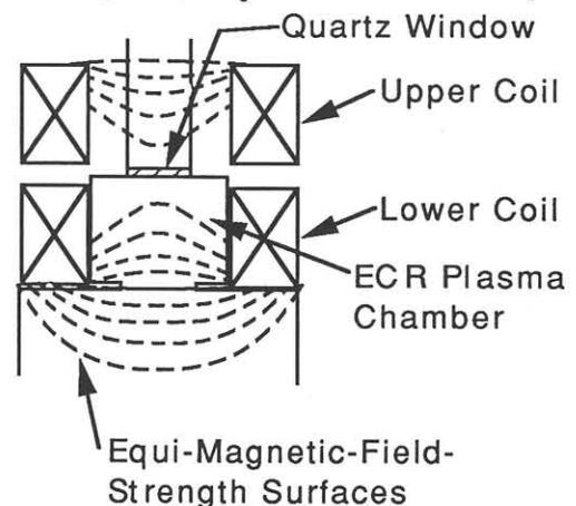
Fig. 1 Magnetic configuration and the equi-magnetic-field-strength surfaces of a standard ECR plasma apparatus.
