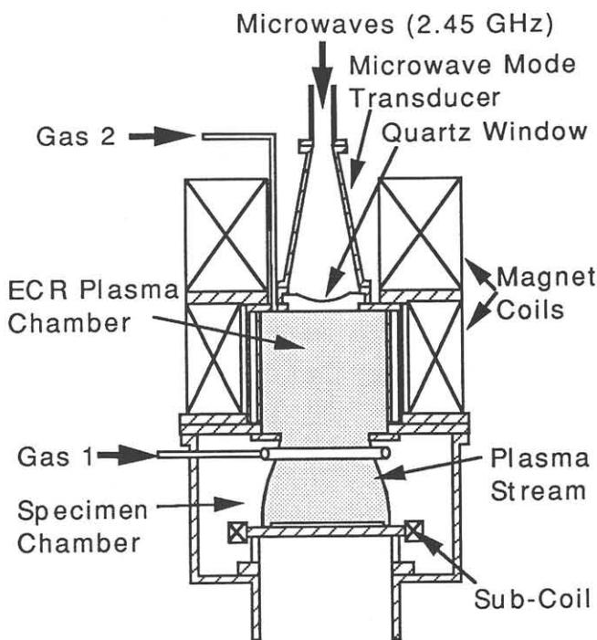
Fig. 5 Novel ECR plasma processing apparatus using the new magnetic configuration.
