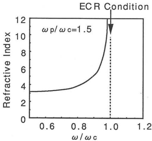
Fig. 2 Dependence of the equivalent refractive index of the plasma frequency. The horizontal axis is the ratio of the microwave frequency  $\omega$  to the cyclotron frequency  $\omega_c$  ( $=eB/m$ ).
