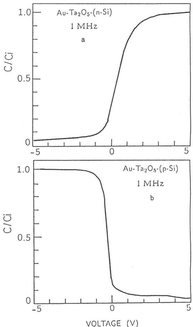
Fig. 2: Well defined capacitance voltage characteristics of Au-Ta<sub>2</sub>O<sub>5</sub>/Si MOS diodes.
