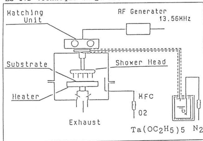
Fig.1 Experimental set-up for plasma enhanced liquid source-CVD (SAMCO model PD240).
