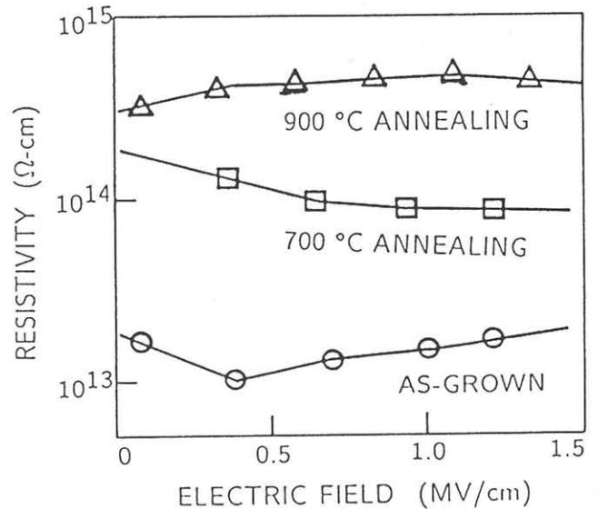
Fig. 4: Effects of rapid thermal annealing on Ta<sub>2</sub>O<sub>5</sub> films resistivity measured as a function of applied electric fields.
