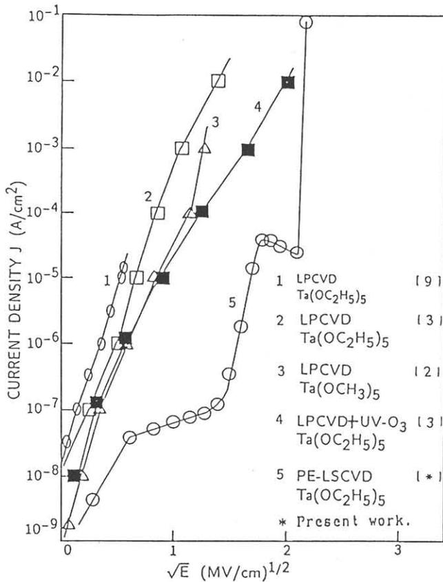
Fig. 3: Current voltage characteristics of Ta<sub>2</sub>O<sub>5</sub>. Our data is compared with those reported for carbon-based liquid sources.
