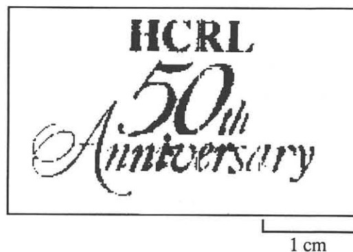
Fig.6 Output image detected by the sensor. The detection time is 0.5 s.
