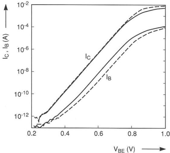
Figure 3: Gummel plot of transistors with As (solid line) and P-doped (dashed line) polysilicon emitter.
