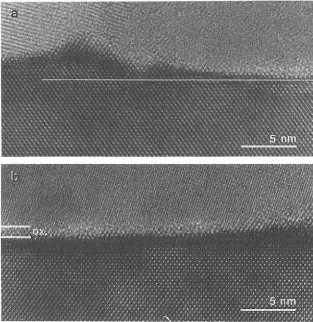
Figure 5: HRTEM of poly-mono interface of As (a) and P-doped (b) polyemitter.
