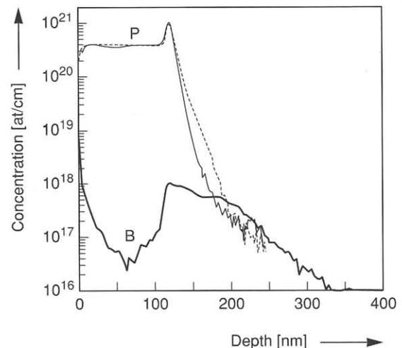
Figure 1: SIMS of P and B, from emitter area, annealed at  $900$  (solid line) and  $975^\circ\text{C}$  (dashed line).
