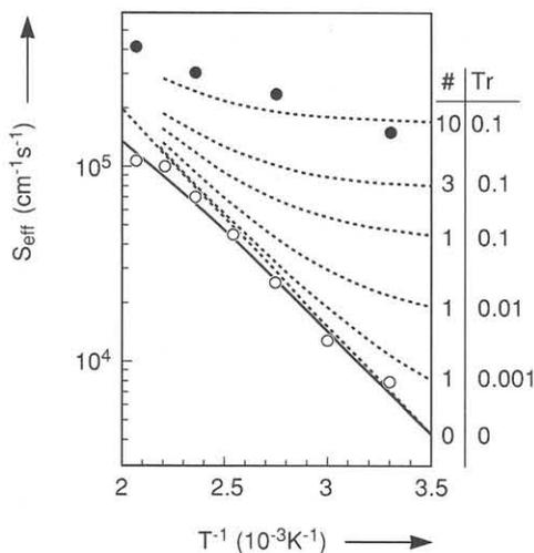
Figure 6: Dashed lines: calculated  $S_{eff}$  as a function of the transparency (Tr) and number of gaps (#). Solid line: eq. 1.
