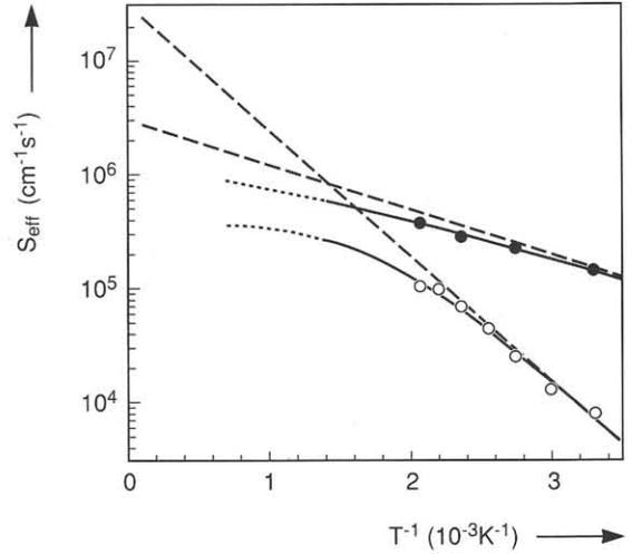
Figure 4:  $S_{eff}$  of As (dots) and P-doped (circles) polyemitter. Solid line: eq. 1, dashed line:  $S_{eff} = v_{tr}$ .
