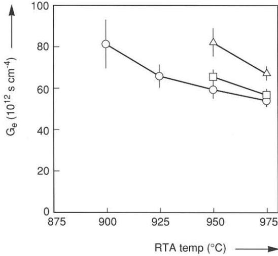
Figure 2: Emitter Gummel number vs. annealing temperatures of P-doped polysilicon emitter. Circles, squares and triangles correspond to base-implantation doses of  $1.2$ ,  $2.4$  and  $3.6 \times 10^{13} \text{cm}^{-2}$ , respectively. Error bars denote variations over the wafers.
