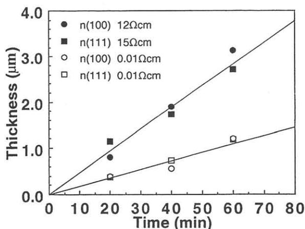
Fig. 3 Porous layer thickness increases linearly with the photo-irradiation time.
