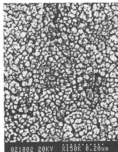
Fig. 6 Surface of the photosynthesized porous layer on n<sup>+</sup>-Si.
