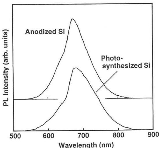
Fig. 5 Comparison of PL spectra between anodization and photosynthesis.
