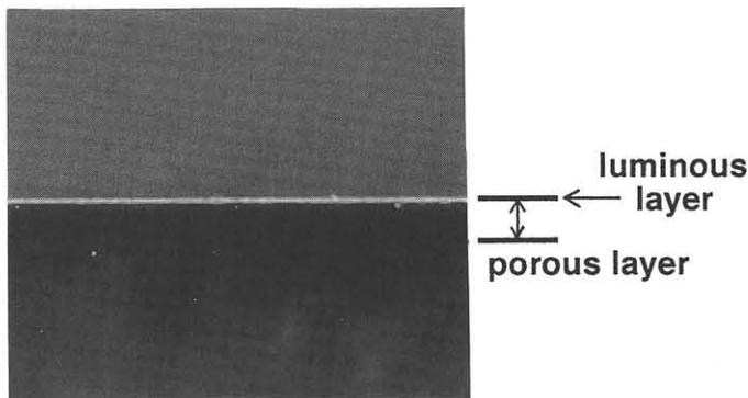
Fig. 1 Cross-sectional PL image of (111)Si anodized for 1h in 25%HF solution. Porous layer is 26 $\mu\text{m}$  thick in this example.
