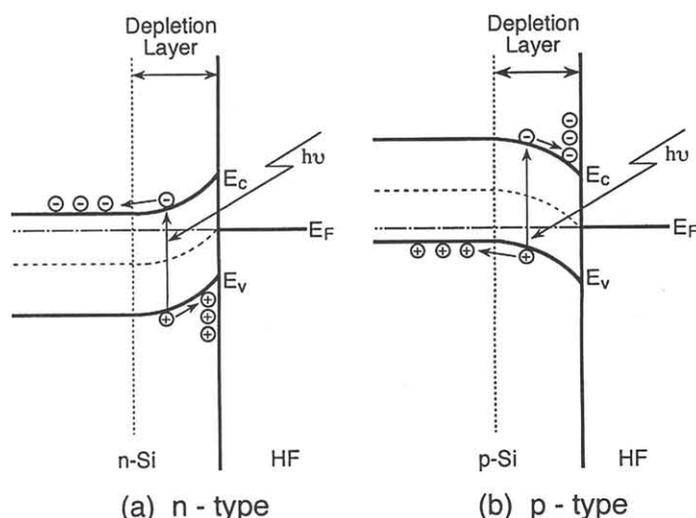
Fig.4 Behavior of Photo-generated holes in the surface depletion layer.
