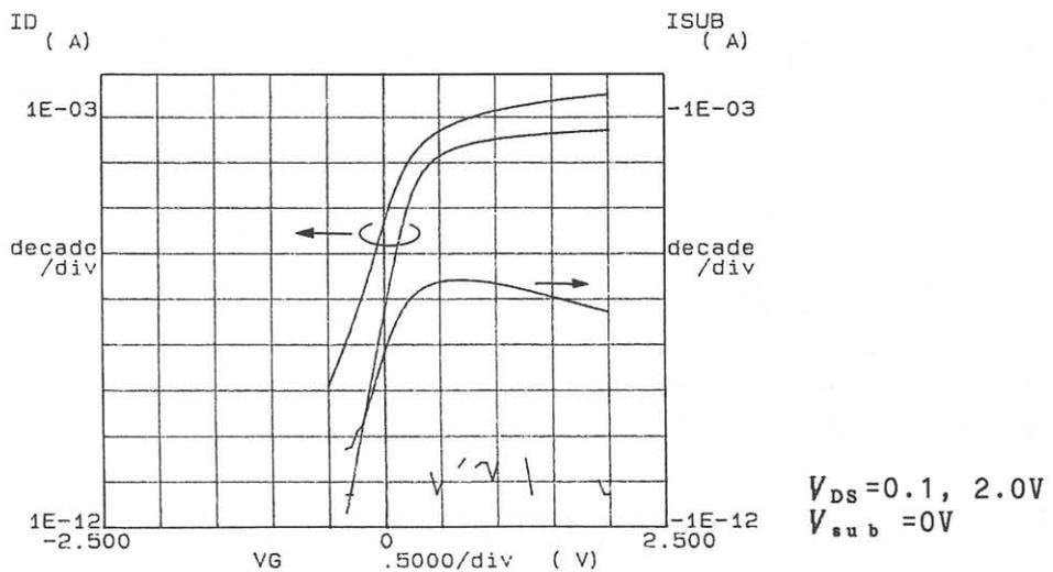
Figure 3.  $I_D$  and  $I_{\text{sub}} - V_{GS}$  characteristics of a transistor with a 150-nm long gate (the same transistor as shown in Figure 2).
