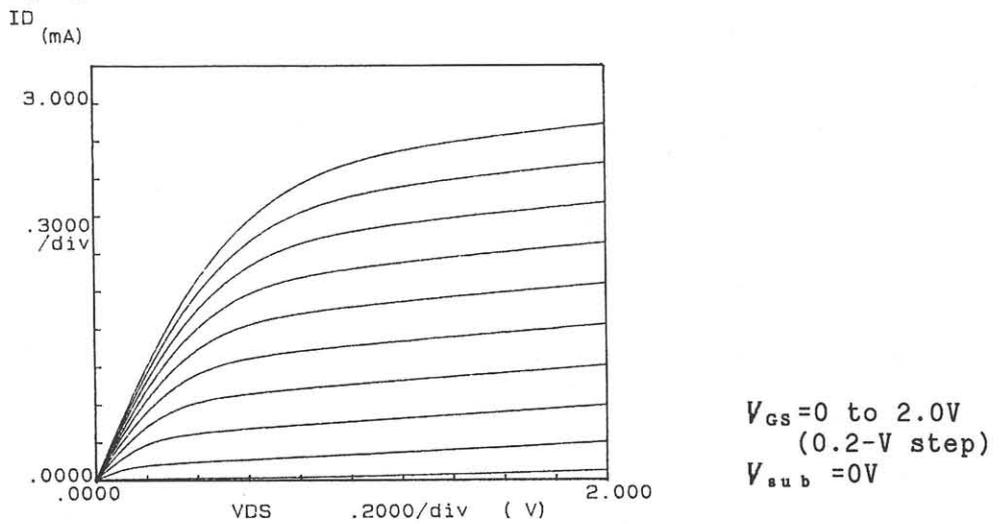
Figure 2.  $I_D - V_{DS}$  characteristics of a transistor with a 150-nm long gate. The sidewall-spacer is 40nm long.  $W=5\mu\text{m}$ ,  $t_{\text{ox}}=5\text{nm}$ , and the channel doping dose is  $3 \times 10^{12}\text{cm}^{-2}$ .
