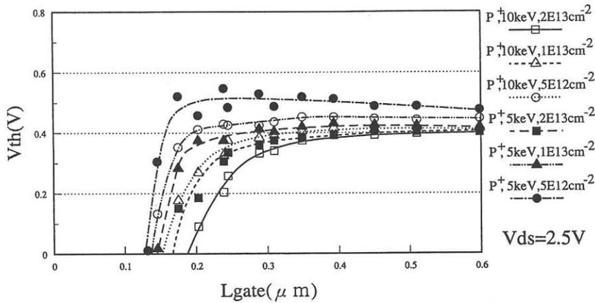
Figure 1. Dependence of threshold voltage on gate length for various LDD-implant conditions.  $W=5\mu\text{m}$ ,  $t_{\text{ox}}=5\text{nm}$ , the sidewall-spacers are 100nm long, and the channel doping dose is  $6 \times 10^{12}\text{cm}^{-2}$ .
