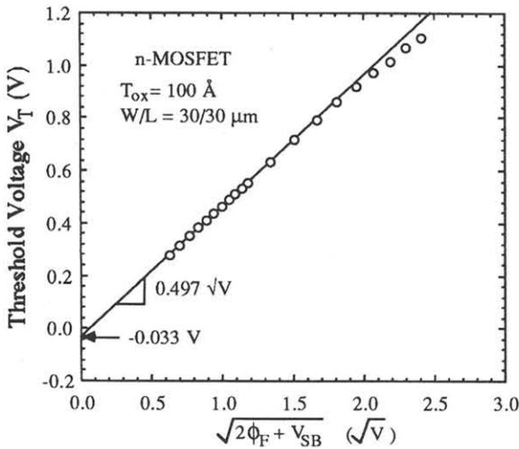
Fig. 1. Body-effect of an n-MOSFET.
