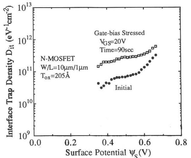
Fig. 5. The energy distribution of interface traps in the band gap for the initial n-MOSFET ( $\bullet$ ) and the gate-bias stressed MOSFET ( $\square$ ).
