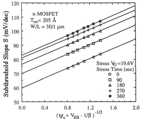
Fig. 4. Increase of the subthreshold slope by the high gate-bias stress, with stress time as a parameter.
