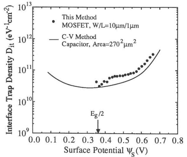
Fig. 3. The energy distribution of interface traps in the band gap for n-MOSFET from the subthreshold slope measurement ( $\bullet$ ) and that for a capacitor from the C-V method ( $-$ ).
