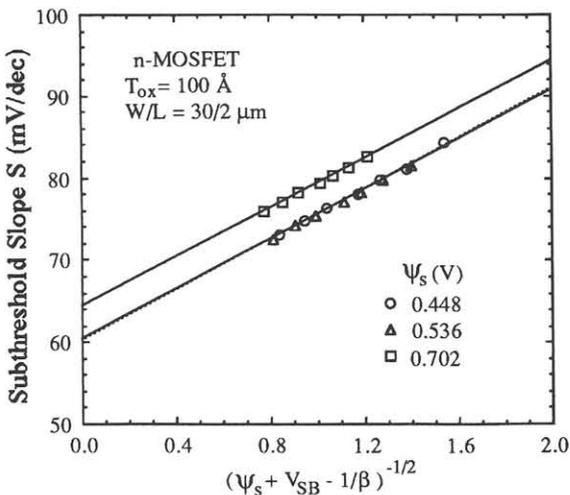
Fig. 2. The subthreshold slope dependence on the substrate bias with surface potential as a parameter.
