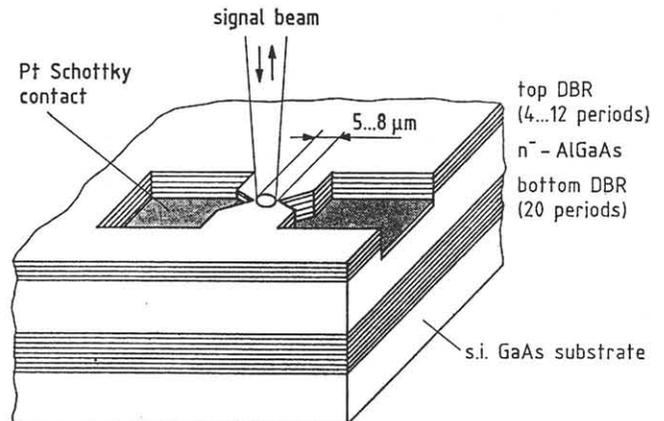
Fig. 1: Design of wavelength selective MSM photodetector with integrated Fabry-Perot resonator.
