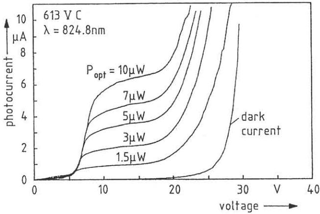
Fig. 2: Current-voltage characteristics at different optical power levels.
