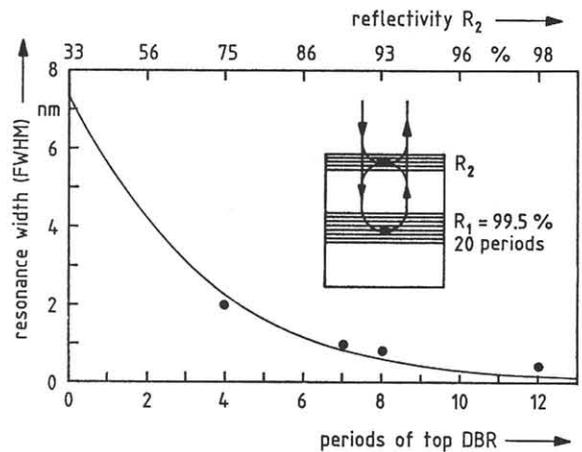
Fig. 4: Resonance width in dependence on the number of periods in the top DBR, exp. (●) and calc. (—) results.
