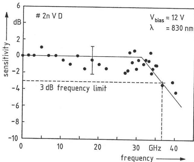
Fig. 5: Frequency characteristics of a resonant MSM photodetector mounted onto a 2.4 mm flange.
