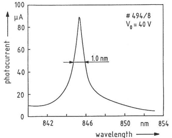
Fig. 3: Photocurrent-wavelength characteristics of a wavelength selective MSM photodetector (top DBR: 7 periods, bottom DBR: 20 periods).
