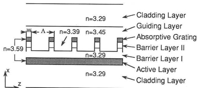
Fig.1. Schematic of the longitudinal cross section of the GC DFB laser having an absorptive grating.
