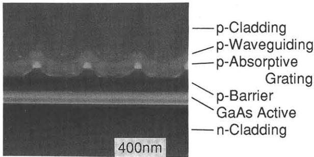
Fig.3. Scanning electron micrograph of the epitaxial layers showing the absorptive grating with a small duty factor ( $\sim 0.15$ ).
