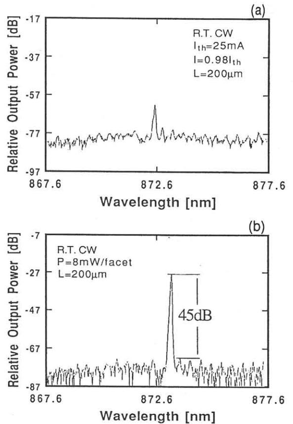
Fig.4. Spectra of the GaAlAs/GaAs GC-DFB laser fabricated (200 $\mu\text{m}$ -long with both facets as cleaved); (a) below threshold and (b) at the output of 8mW.
