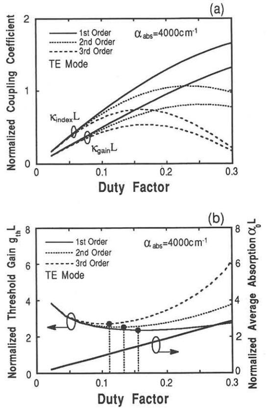
Fig.2. (a) Normalized index- and gain-coupling coefficients versus the duty factor of the grating; (b) normalized averaged absorption ( $\alpha_0L$ ) and threshold gain ( $g_{th}L$ ) versus duty factor of the grating.
