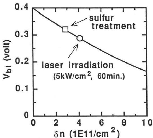
Fig. 3. The relationship between the built-in potential and the increase in carrier density.
