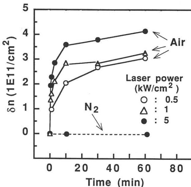
Fig. 2. Carrier density increase due to laser irradiation. The horizontal axis indicates laser irradiation time.
