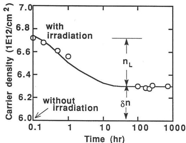
Fig. 1. Typical behavior of carrier density observed in Hall devices with in-air laser irradiation. The horizontal axis indicates the elapsed time after the devices are placed in darkness.  $n_L$  originates in photoexcited carriers and  $\delta n$  is the real increase in carrier density eliminating the influence of the photoexcited carriers.
