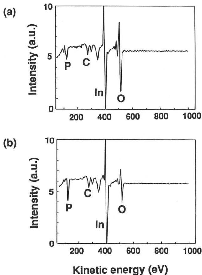
Fig. 4. AES spectra of InP. (a) With laser irradiation ( $5 \text{ kW/cm}^2$ , 60 min.). (b) Without laser irradiation.
