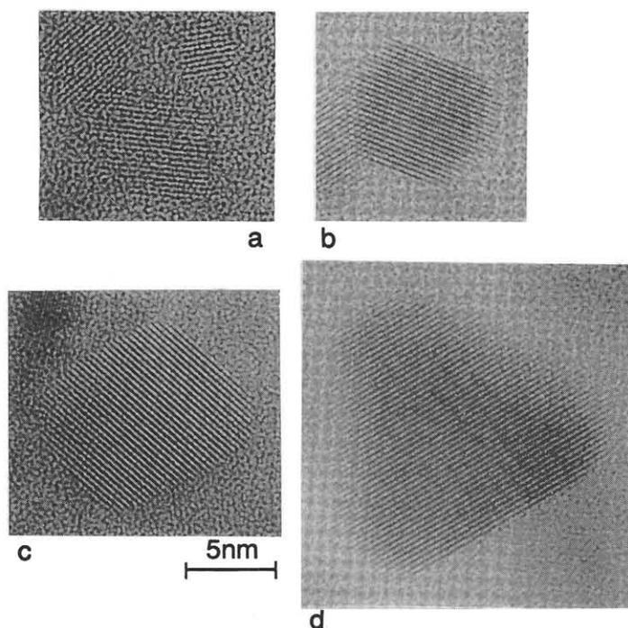
Fig. 3 Morphology of  $\mu\text{-Ge}$  formed in a SiO<sub>2</sub> glassy matrix.
