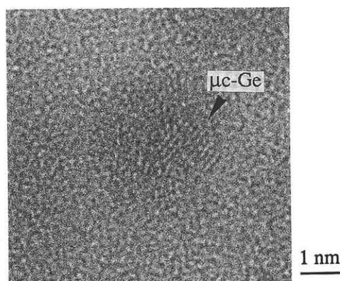
Fig. 2 Very small  $\mu\text{-Ge}$  formed in Ge dense portion (dark portion) at 300°C annealing.
