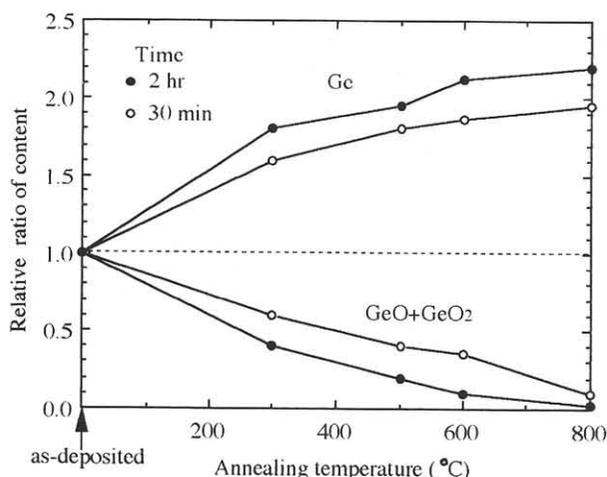
Fig. 1 Relative ratio of each content obtained from XPS data. The ratio is normalized by the content of the as-deposited sample.
