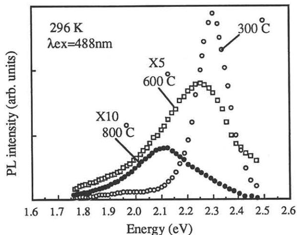
Fig.4 PL spectrum for the sample annealed at each temperature.
