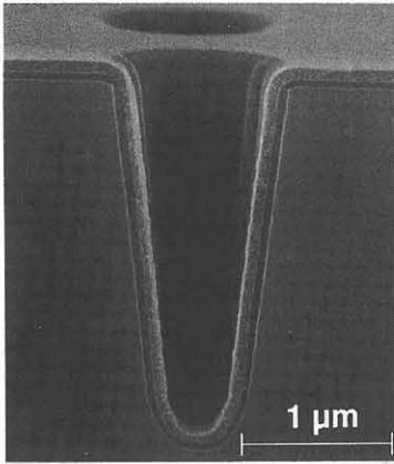
Fig. 2 SEM photograph of a trench partially filled with boron doped silicon film deposited from  $\text{Si}_2\text{H}_6/\text{B}_2\text{H}_6$  mixture at  $350^\circ\text{C}$ .
