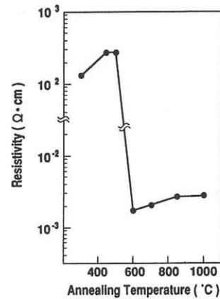
Fig. 6 Resistivity as a function of annealing temperature, this film was deposited using  $\text{Si}_2\text{H}_6/\text{B}_2\text{H}_6$  at  $350^\circ\text{C}$ .
