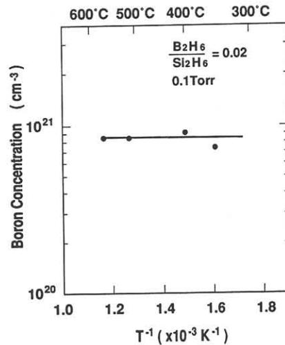
Fig. 3 The variation in boron concentration as a function of substrate temperature.
