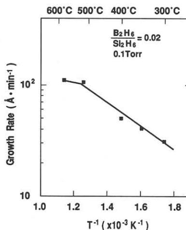
Fig. 1 Growth rate as a function of substrate temperature with the  $\text{Si}_2\text{H}_6/\text{B}_2\text{H}_6$  mixture.
