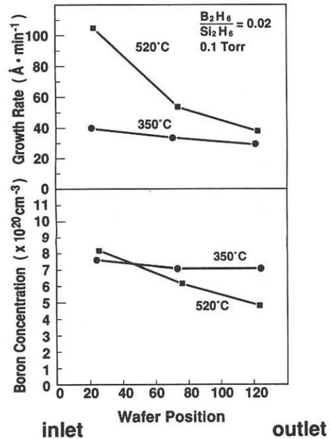
Fig. 4 The distributions in boron concentration and growth rate among wafers in a reactor at deposition temperatures of  $520^\circ\text{C}$  and  $350^\circ\text{C}$ .
