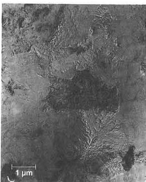
Fig. 5 TEM photograph showing the grain structure of boron-doped polysilicon annealed at  $600^\circ\text{C}$  for 60 minutes.
