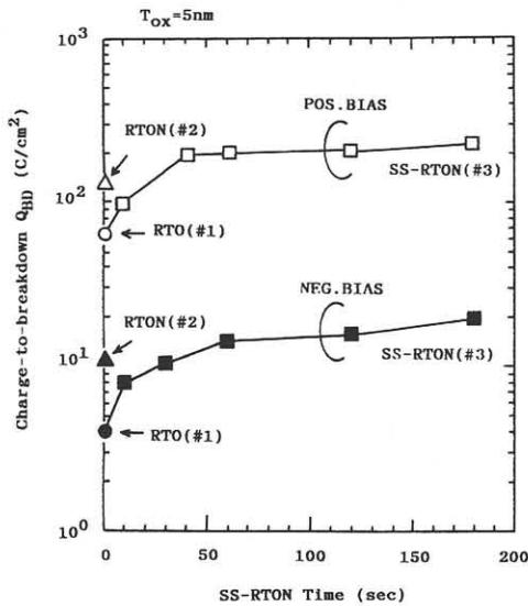
Fig.4 The dependence of SS-RTON time on the charge-to-breakdown.
