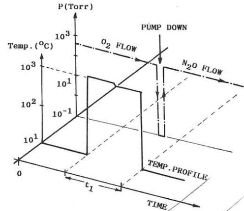
Fig.1 Temperature and gas flow profiles for SS-RTON process.
