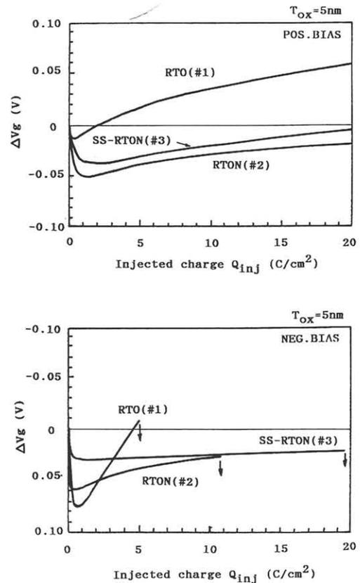
Fig.2 Gate voltage shifts against injected charge for samples (#1)-(#3) @  $J_{ox} = \pm 100 \text{ mA/cm}^2$ .
