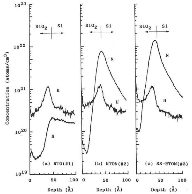
Fig.5 SIMS depth profiles of N and H atoms in samples (#1)-(#3).
