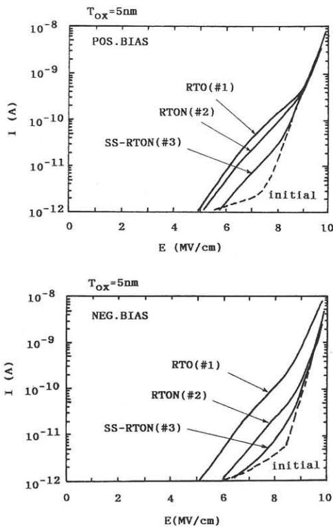
Fig.3 Leakage currents through samples (#1)-(#3) @ $Q_{inj}=5C/cm^2$ .
