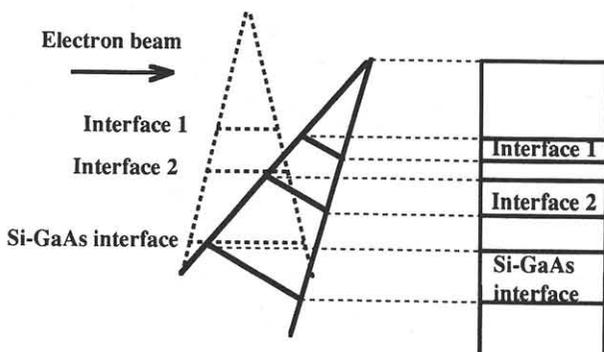
Fig. 2(a) Inclined XTEM shown schematically.
