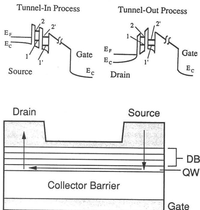
Figure 1: The schematic cross section of our transistor structure. The energy band diagrams at the 'tunneling-in' and the 'tunneling-out' junctions are also shown, where  $E_C$  is the conduction band minimum,  $E_F$  is the Fermi level, 1, 2 depicts the lowest two subband levels in the DB RT structures, and 1', 2' depicts the lowest two subband levels in the QW.
