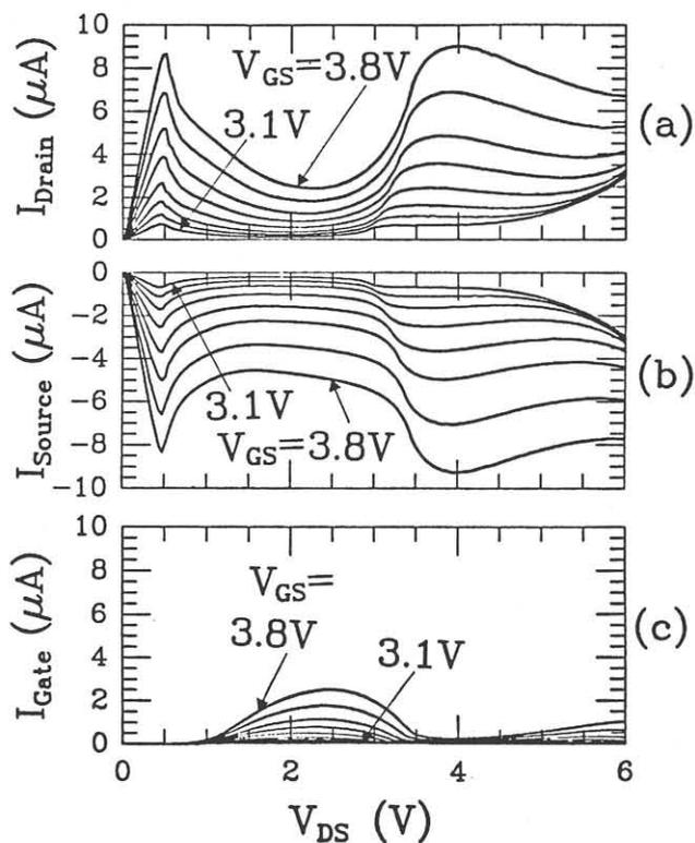
Figure 2: DC I-V characteristics of our transistor at 77K, where (a)  $I_{Drain}$  versus  $V_{DS}$ , (b)  $I_{Source}$  versus  $V_{DS}$ , and (c)  $I_{Gate}$  versus  $V_{DS}$ , are shown. The  $V_{GS}$  is stepped evenly from 3.1V to 3.8V.
