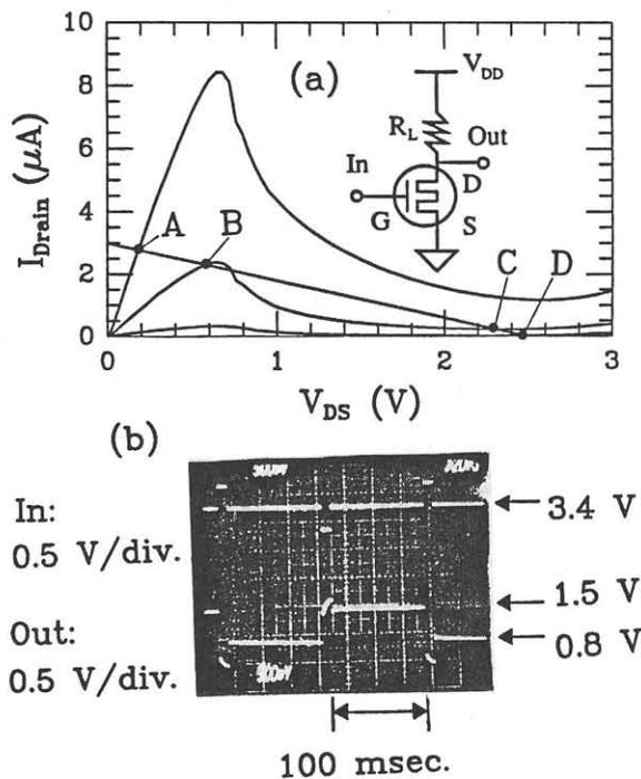
Figure 3: (a) DC I-V characteristics of our transistor at 77K, and the circuit configuration and the load lines are also shown in the inset. The power supply voltage  $V_{DD}$  is 2.47V. The operating points discussed in the context are labeled as A, B, C, and D. (b) Waveforms of input ( $V_{GS}$ ) and output voltage signals.
