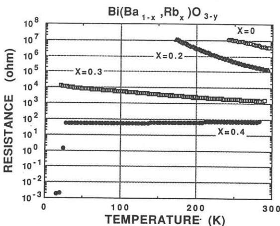
Fig. 6  $R(T)$  as a function of Rb composition ratio.
