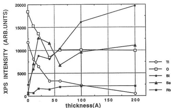
Fig. 4 XPS intensity as a function of average thickness of BRBO on STO(100).
