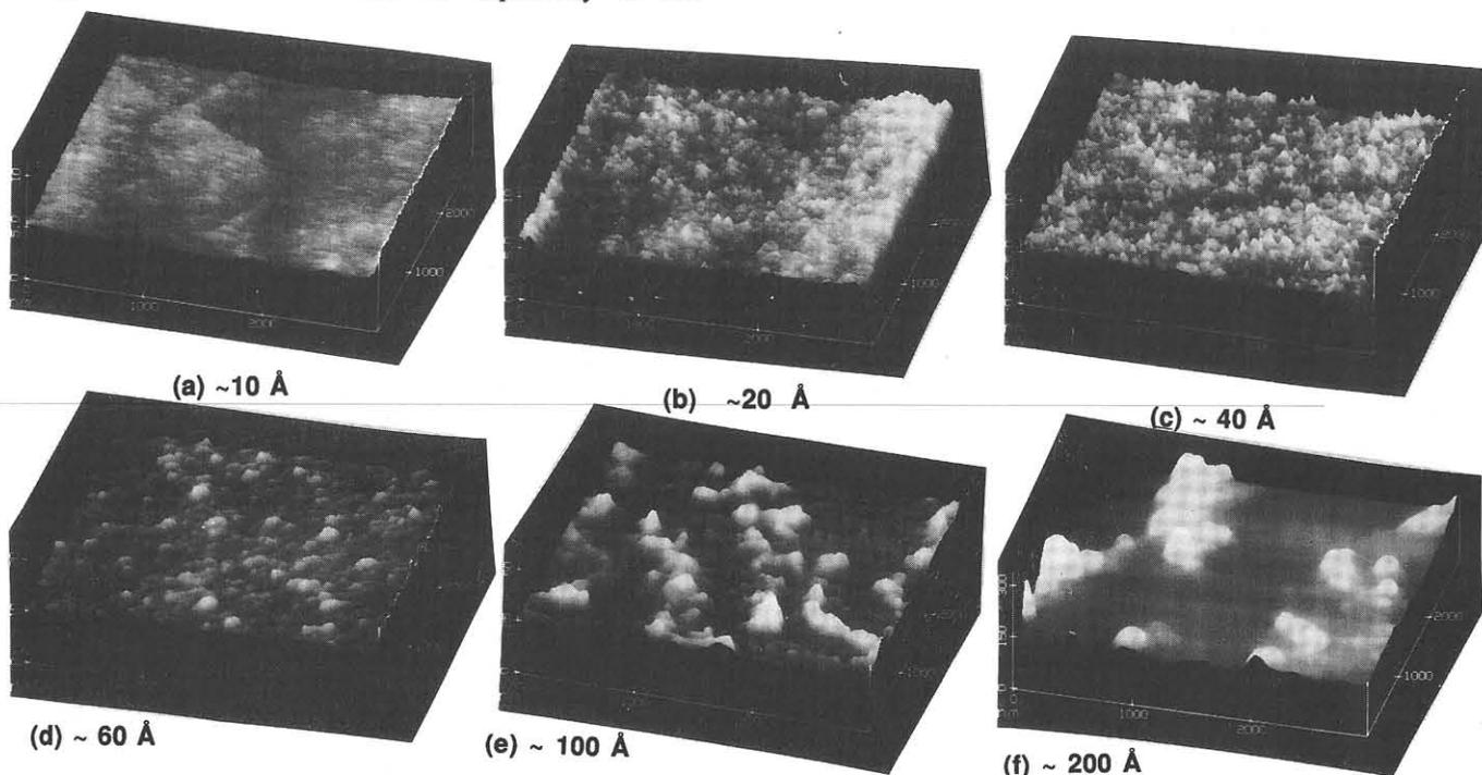
Fig. 3 AFM observation of BRBO during BRBO film growth.
