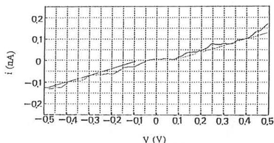
Fig.2 The current-voltage characteristic of 1D array. Coulomb blockade is observed and the first step in the  $i$ - $v$  curve occurs at 150 mV. After bringing the tip to the tunnel regime (the bias voltage is 1V (sample positive) and set point current is 0.2 nA), the feedback was cut, the bias voltage was ramped and the current was measured.
