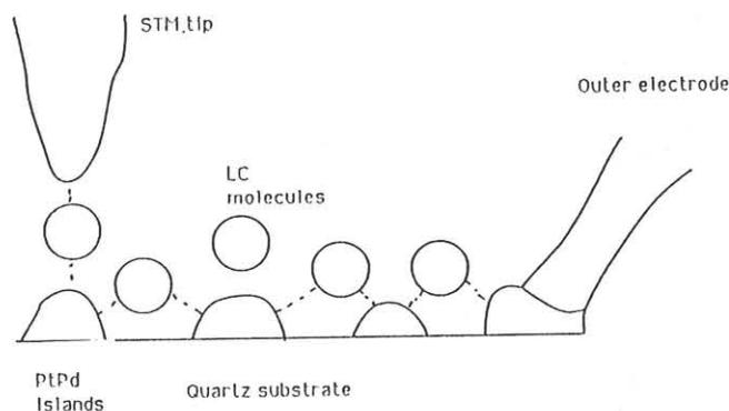
Fig.1 A schematic picture of the electronic circuit realized by molecule. PtPd islands were formed on a quartz substrate. LC molecules were put on this substrate and molecules occupy the position between islands.
