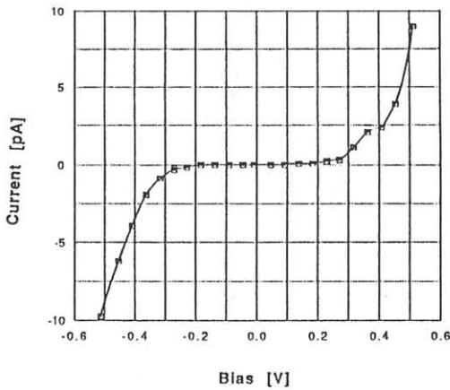
Fig.3 The calculated  $i$ - $v$  curve using SETCAD program. The number of tunnel junctions is 14. There is a Coulomb gap and it agrees well with the experimental result (Fig.2).
