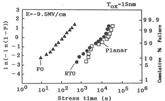
Fig.4 Cumulative TDDDB characteristics for BG-type and planar-type MOS devices.
