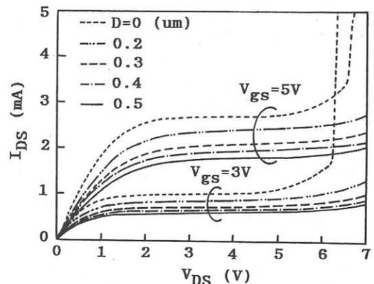
Fig.5 The experimental I<sub>ds</sub>-V<sub>ds</sub> of BG-MOSFET with gate length of 1.0 μm.
