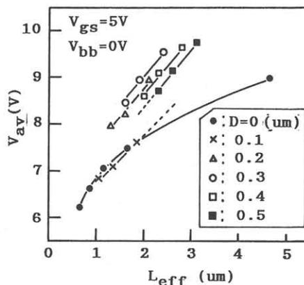
Fig.6 The  $V_{av}$ - $L_{eff}$  characteristics as a function of trench depth.
