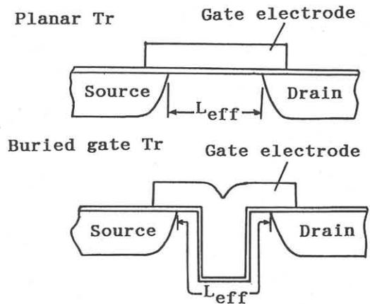
Fig.2 Schematic drawing of planar-type and BG-MOSFETs.
