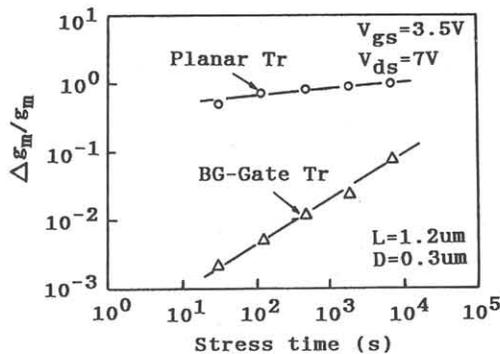
Fig.8 The  $\Delta g_m/g_m$  characteristics for planar and BG-MOSFETs.
