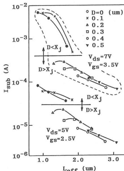
Fig.7 The experimental  $I_{sub}$ - $L_{eff}$  characteristics of BG-MOSFETs.
