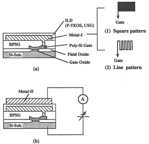
Fig.1 (a) Cross sectional structure of test sample for TDDDB and FDDDB measurements. (b) Cross sectional structure of test sample for V-I characteristic measurements.
