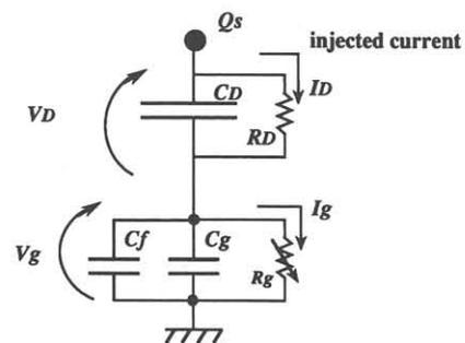
Fig.4 Model of charge injection through interlayer dielectric :  $Q_s$  was surface charge on dielectric.  $C_D$ ,  $C_f$  and  $C_g$  were capacitors of interlayer dielectric, field oxide and gate oxide, respectively.  $V_D$  and  $V_g$  were voltage of dielectric and gate.  $R_D$  and  $R_g$  were a resistance of dielectric and gate oxide.
