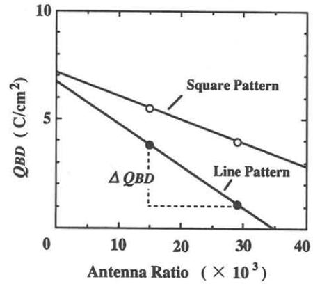
Fig.5 Dependence of  $Q_{BD}$  on antenna ratio in the case of P-TEOS.
