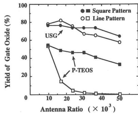
Fig.3 Dependence of gate oxide breakdown on antenna ratio and materials of interlayer dielectric.
