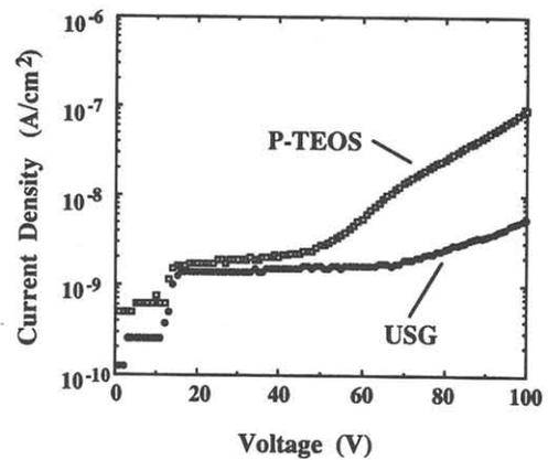
Fig.6 Current density versus voltage for the test sample in Fig.1-(b)
