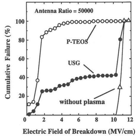
Fig.2 Breakdown field of gate oxide before and after plasma irradiation
