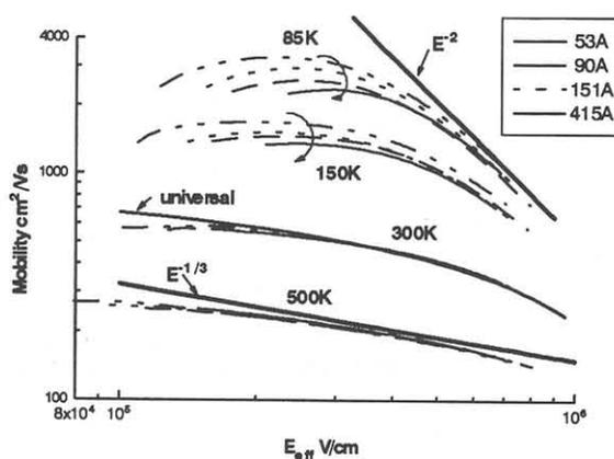
Fig. 1 The effective electron mobility versus effective field measured from 85K to 500K for nMOSFETs.  $N_B = 2.4 \times 10^{16} \text{cm}^{-3}$ ,  $W/L = 100 \mu\text{m}/28 \mu\text{m}$ , and  $T_{ox}$  ranges from 53Å to 415Å. Peak mobility shows oxide thickness dependence.
