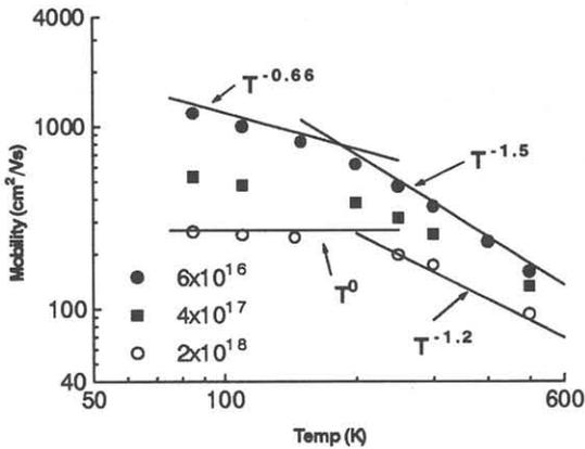
**Fig. 5** Electron mobility measured at different temperatures from moderate to very highly doped substrates emphasizing the temperature dependencies of phonon, coulomb, and surface roughness scattering. Device parameters are  $N_B = 6 \times 10^{16} \text{ cm}^{-3}$  to  $1.7 \times 10^{18} \text{ cm}^{-3}$ ,  $T_{ox} = 145 \text{ \AA}$ , and  $W/L = 100 \text{ μm} / 28 \text{ μm}$ .
