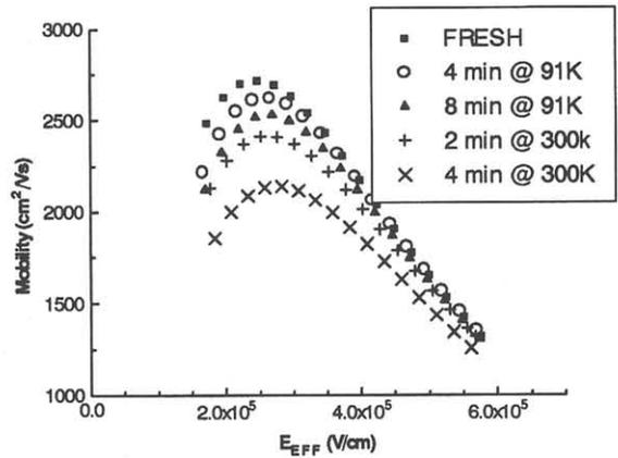
**Fig. 7** Electron mobility measured at 91K for Substrate Hot Electron stress at 91K and 300K. The device parameters are  $N_B = 2.4 \times 10^{16} \text{ cm}^{-3}$ ,  $T_{ox} = 90 \text{ \AA}$ , and  $W/L = 100 \text{ μm} / 10 \text{ μm}$ .
