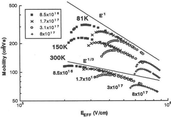
**Fig. 4** Hole mobility versus effective electric field for devices over the temperature range 81K to 300K.  $N_B = 8.5 \times 10^{16} \text{ cm}^{-3}$  to  $8 \times 10^{17} \text{ cm}^{-3}$ .  $T_{ox} \approx 110 \text{ \AA}$  and  $W/L = 70 \text{ μm} / 20 \text{ μm}$ .
