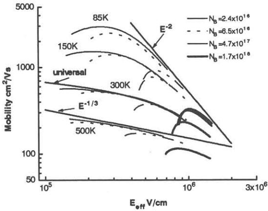
**Fig. 3** Effective mobility of electrons versus effective electric field for devices over the temperature range 85K to 500K with  $N_B$  varying from  $2.4 \times 10^{16} \text{ cm}^{-3}$  to  $1.7 \times 10^{18} \text{ cm}^{-3}$ . All of the devices had  $T_{ox} \approx 145 \text{ \AA}$  and  $W/L = 100 \text{ μm} / 28 \text{ μm}$ .
