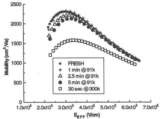
**Fig. 8** Electron mobility measured at 91K for Substrate Hot Electron stress at 91K and 300K. The device parameters are  $N_B = 6 \times 10^{16} \text{ cm}^{-3}$ ,  $T_{ox} = 145 \text{ \AA}$ , and  $W/L = 100 \text{ μm} / 10 \text{ μm}$ .
