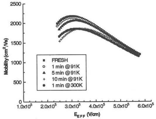
**Fig. 6** Electron mobility measured at 91K for Substrate Hot Electron stress at 91K and 300K. The device parameters are  $N_B = 6 \times 10^{16} \text{ cm}^{-3}$ ,  $T_{ox} = 94 \text{ \AA}$ , and  $W/L = 100 \text{ μm} / 10 \text{ μm}$ .
