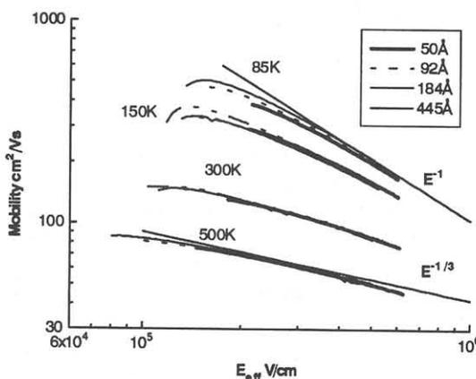
Fig. 2 The effective hole mobility versus effective field measured from 85K to 500K for pMOSFETs. The device parameters are  $N_B = 3.5 \times 10^{16} \text{cm}^{-3}$ ,  $W/L = 100 \mu\text{m}/28 \mu\text{m}$ , and  $T_{ox}$  ranges from 50Å to 445Å.
