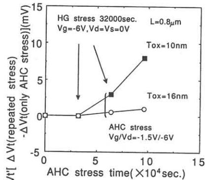
Fig.4.  $\Delta Vt'$  [ $\Delta Vt$ (repeated stress) -  $\Delta Vt$ (only AHC stress)] dependent of gate oxide thickness under repeated stress : at gate oxide of 10nm vs at gate oxide of 16nm
