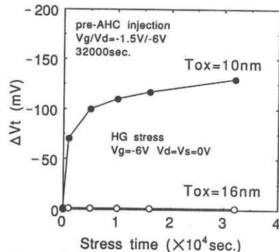
Fig.5.  $\Delta Vt$  under HG stress after AHC injection : at gate oxide of 10nm vs at gate oxide of 16nm
