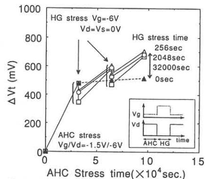
Fig.1.  $\Delta V_t$  as a function of HG stress time (HG stress is high gate and low drain voltage stress) : under repetition of AHC stress and HG stress vs only AHC stress
