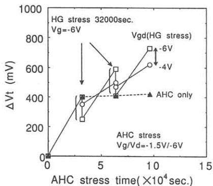
Fig.6.  $\Delta V_t$  dependent of  $V_{gd}(V_{gs})$  under HG stress
