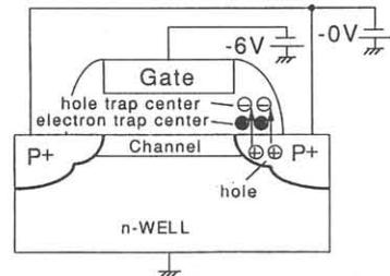
Fig.8. Model of hole injection into the new trap centers in the gate oxide above the drain under high gate and low drain voltage stress
