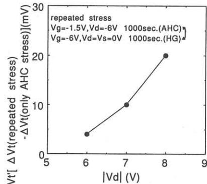
Fig.3.  $\Delta Vt'$  [ $\Delta Vt$ (repeated stress) -  $\Delta Vt$ (only AHC stress)] dependent of Vd under AHC stress
