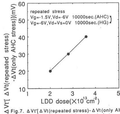
Fig.7.  $\Delta V_t$  [ $\Delta V_t$ (repeated stress)- $\Delta V_t$ (only AHC stress)] dependent of LDD dose under repeated stress
