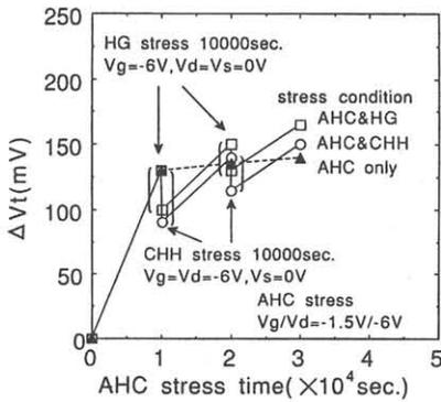
Fig.2.  $\Delta Vt$  dependent of stress conditions : under AHC&HG stress vs AHC&CHH stress
