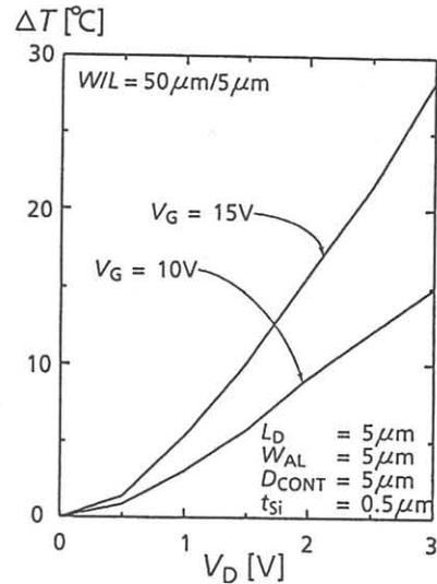
Fig.6 Temperature rise with increasing the drain voltage.
