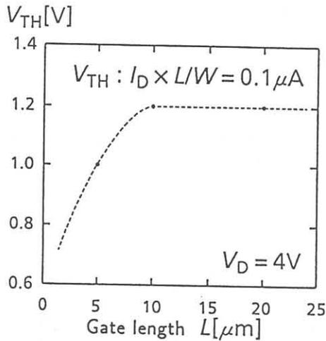
Fig.3 Gate length dependence of threshold voltage.
