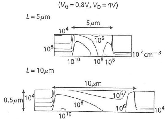
Fig.5 Two dimensional distribution of hole concentration.
