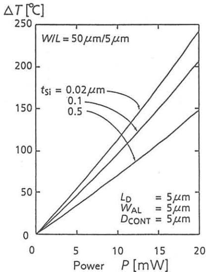
Fig.9 Temperature rise vs. power consumption changing the poly-Si thickness.
