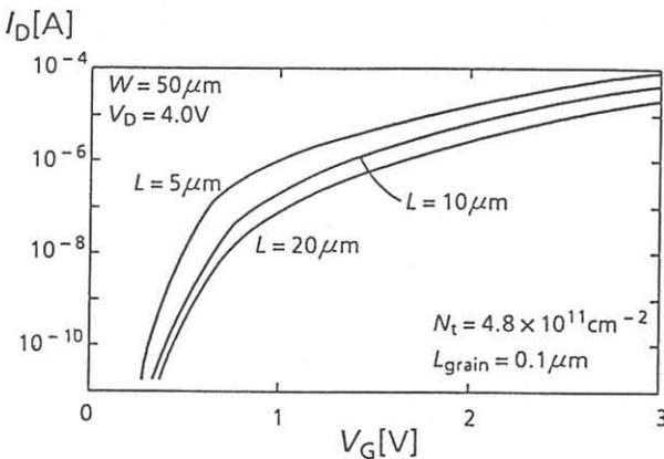
Fig.4 Subthreshold characteristics.
