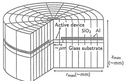
Fig.2 Mesh structure.
