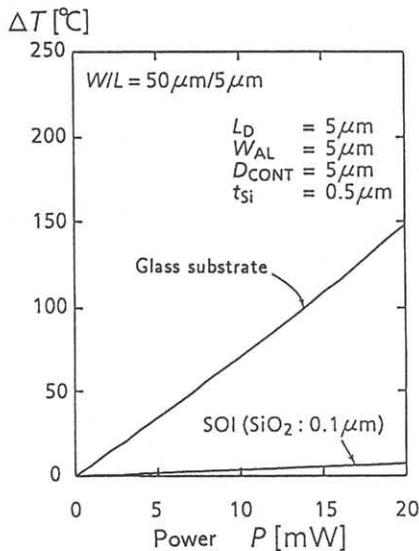
Fig.8 Temperature rise vs. power consumption changing the substrate material.
