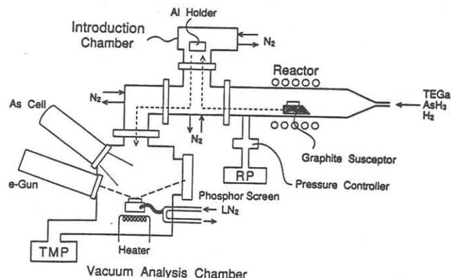
Fig. 1. Schematic illustration of the MOCVD system.
