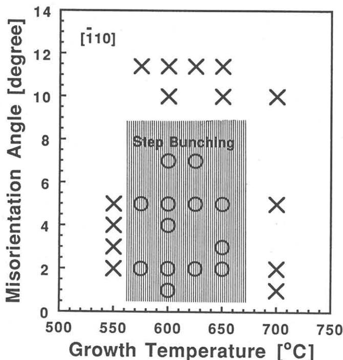
Fig. 3. Phase diagram of the step structure determined by STM and AFM. The growth conditions for which multisteps with more than 3-ML height were observed are considered as step bunching conditions. The circles represent step bunching observed and the crosses represent the absence of step bunching.
