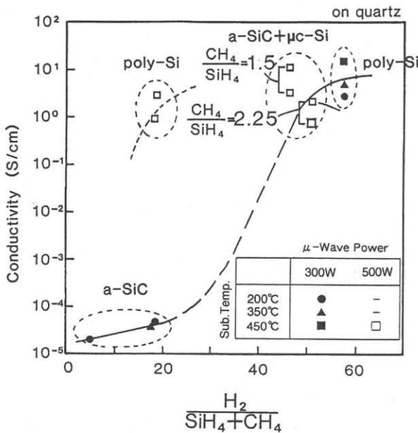
Fig.1 Film conductivity characteristics for various deposition conditions. ( $\text{SiH}_4\text{-CH}_4$  gas system, 1%  $\text{PH}_3$  doped)
