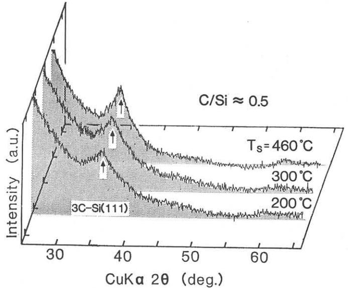
Fig.2 Substrate temperature dependence of X-ray diffraction patterns. ( $\text{Si}(\text{CH}_3)_2\text{H}_2$  gas system,  $\mu$ -wave power = 900W)
