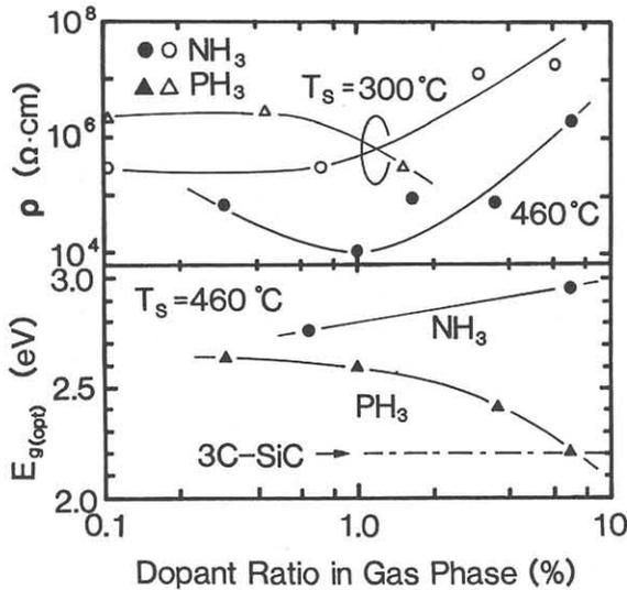
Fig.4 Electrical resistivity and optical energy bandgap of  $\mu\text{c-SiC}$  films as a function of dopant ratio in gas phase.
