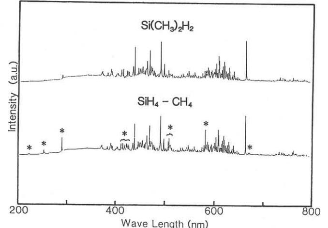
Fig.3 Optical emission spectra of ECR plasma for  $\text{SiH}_4\text{-CH}_4$  and  $\text{Si}(\text{CH}_3)_2\text{H}_2$  gas system. Emission peaks relating to Si and SiHn are marked by \*.
