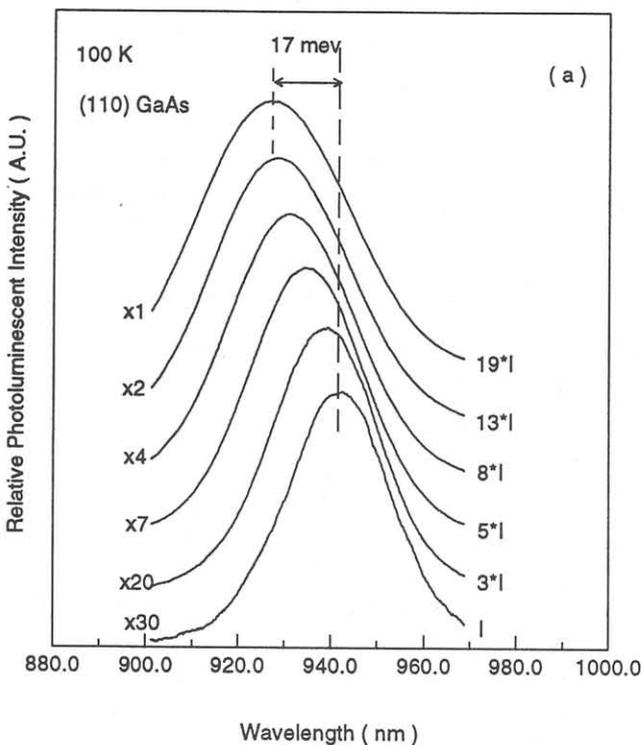
Fig. 1 Photoluminescence spectra of  $\text{In}_{0.2}\text{Ga}_{0.8}\text{As}/\text{GaAs}$  multiple quantum well structures as a function of excitation intensity for layers on (a) (110) and (b) (100) GaAs substrates.
