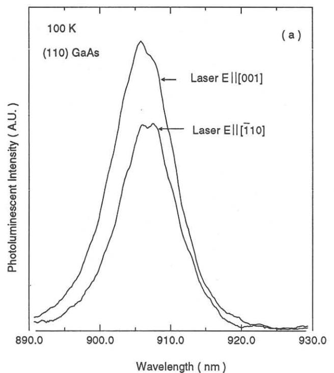
Fig. 2 Photoluminescence spectra of  $\text{In}_{0.2}\text{Ga}_{0.8}\text{As}/\text{GaAs}$  single quantum well structures grown on (a) (110) GaAs and (b) (100) GaAs. The polarization of the excitation source is aligned along two primary crystallographic orientations.
