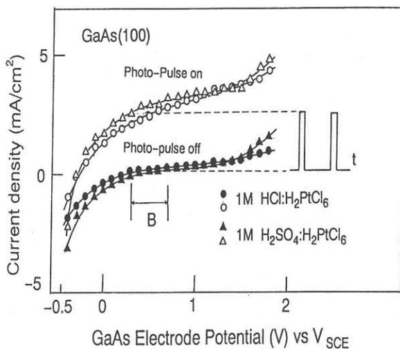
Fig. 2 The current-potential(I-V) curves of n-GaAs(100) electrodes under the illumination by the photo-pulse.
