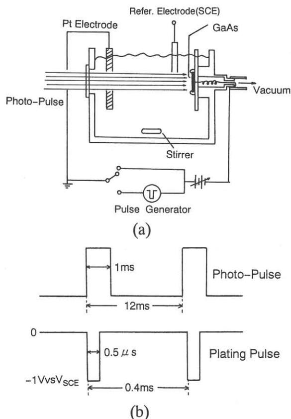
Fig. 1 (a) Experimental setup of the *in-situ* electrochemical processes and (b) photo-pulse and electric plating waveform for plating-pulse.
