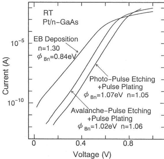
Fig. 5 Forward current-voltage (I-V) characteristics of Pt/GaAs Schottky diodes fabricated by the three kinds of process.
