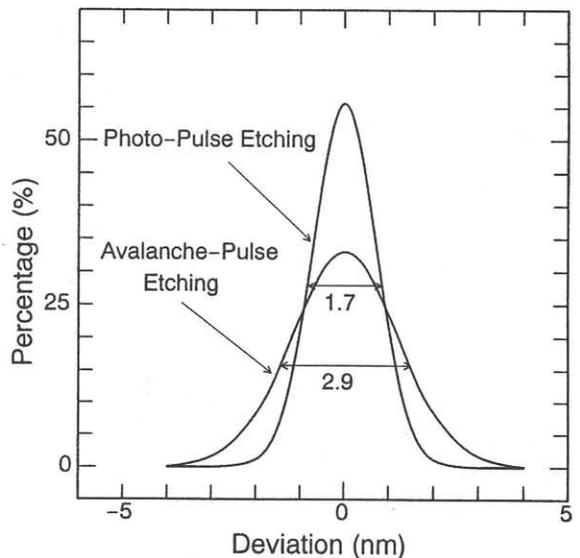
Fig. 3 The histograms of the deviations from the mean height on the etched surfaces, determined by atomic force microscope(AFM).
