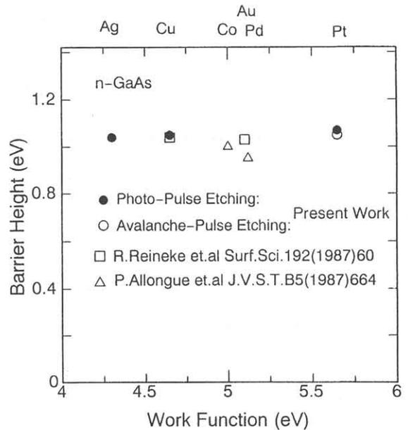
Fig. 6 Schottky barrier height of metal/GaAs contacts by electrochemical processes. The barrier height were determined from I-V measurement, taking account of image force correction of +0.04 eV.
