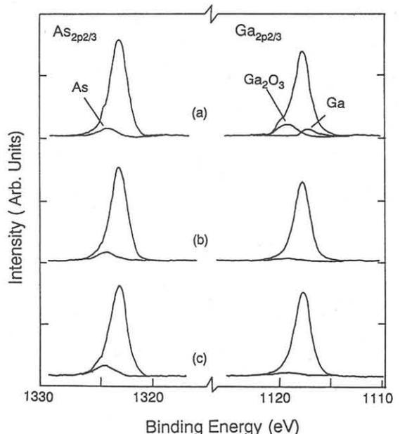
Fig. 4 XPS spectra at the Pt/GaAs interfaces formed by:(a)EB deposition, (b)the pulse-etching electrochemical process and (c)the photo-pulse electrochemical process.
